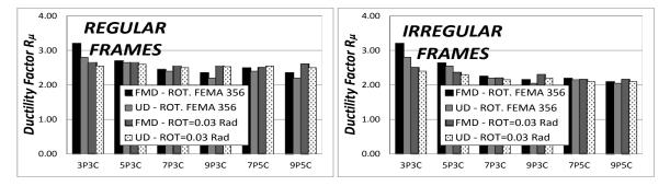
**Figure 4.7.** Ductility Reduction factor  $R_{\mu}$
