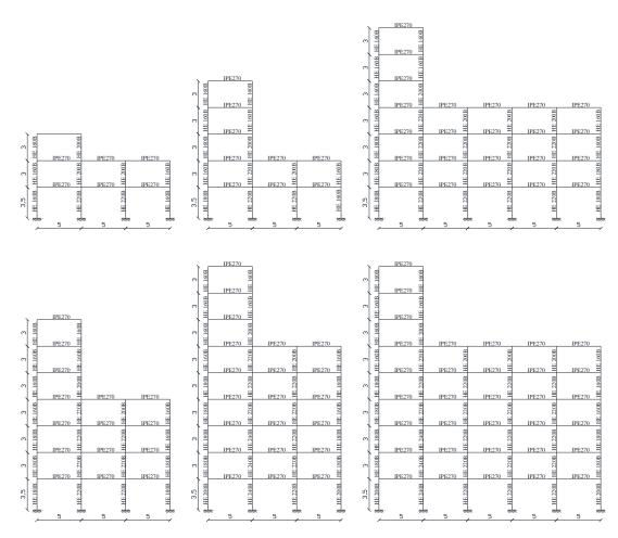
Figure 4.2. Study cases: irregular in elevation moment resisting frame structures.
