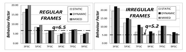
Figure 4.8. Behaviour Factor. Plastic rotation defined according to FEMA
