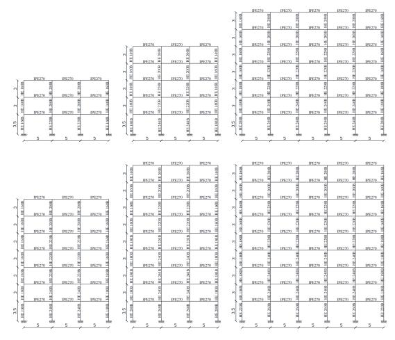
Figure 4.1. Study cases: regular in elevation moment resisting frame structures.
