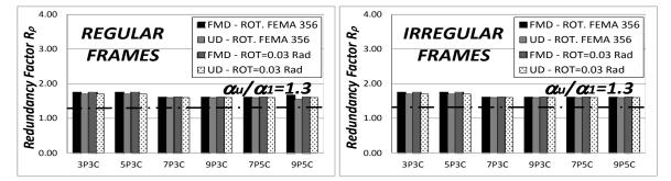
**Figure 4.6.** Redundancy Reduction factor  $R_{\rho}$
