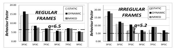
**Figure 4.9.** Behaviour Factor. Ultimate plastic rotation  $\theta_u$ =0.03 rad
