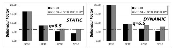
Figure 4.11. Behaviour Factor for frames designed with and without the local ductility criterion ( $N/N_{PL} < 0.3$ )
