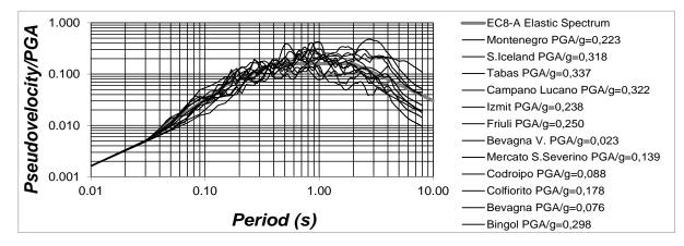
Figure 4.3. Ground motion response spectra and Eurocode 8 elastic response spectrum
