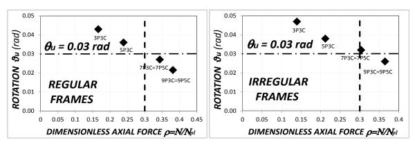
Figure 4.10. Ultimate plastic rotation in base columns
