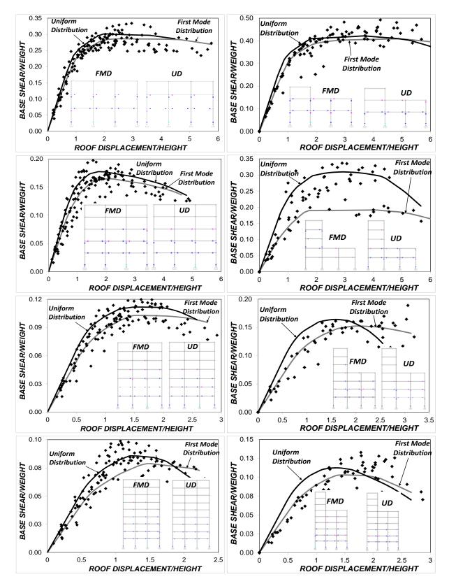
Figure 4.4. Base shear versus roof displacement. Pushover Analysis versus Incremental Dynamic Analysis
