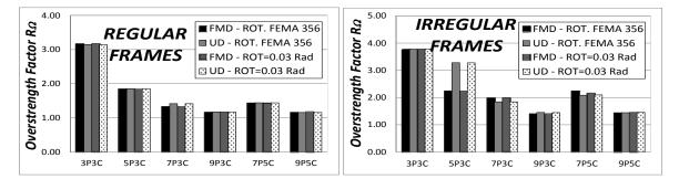
**Figure 4.5.** Overstrength Reduction factor  $R_{\Omega}$
