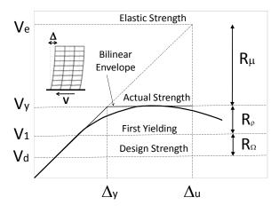
Figure 3.1. Base shear versus roof displacement relationship
