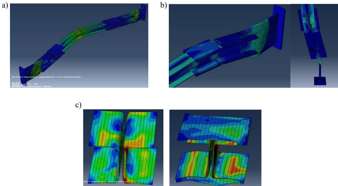
**Figure 7.** a) Brace overall buckling in the first cycle with 12 mm welded outer plates and no gaps; b) Local buckling of the fuse due to slippage of the LBRS ; and c) Von Mises stresses due to flexure in the channels and deformation of the weak 6mm-thick LBRS upon second occurrence of buckling.
