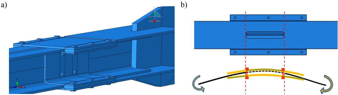
**Figure 9.** a) Channel webs bolted together through the brace web; b) Channels resisting bending moments.
