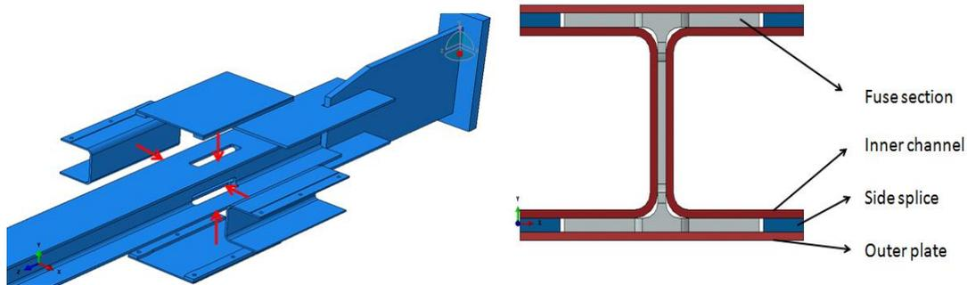
**Figure 5.** Proposed fuse local buckling restraining mechanism.
