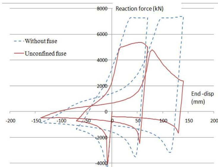
**Figure 4.** Axial load-deformation response of the brace without fuse and with unconfined fuse.
