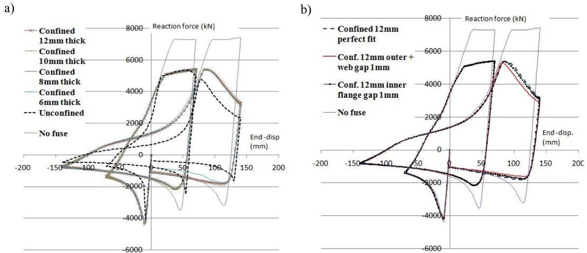
**Figure 6.** Axial load-deformation response of the brace with confined fuses: a) Influence of the thickness of the outer plates (fuse with perfect fit); b) Influence of gaps between components.
