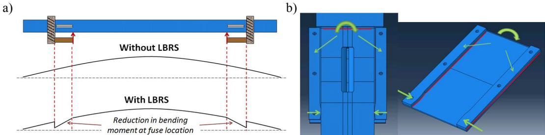
**Figure 10.** a) Brace plan view with bending moment demand on the brace without and with LBRS; b) Moment resisted by the outer plates by the welded connection and transverse contact bearing.
