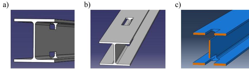
**Figure 1.** Ductile fuse for W-shape bracing members (Vincent 2008):
