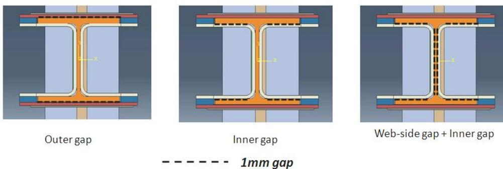
**Figure 8.** Gap conditions considered due to variations in cross-section dimensions
