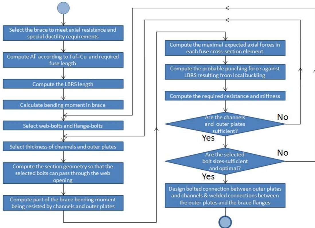
**Figure 11.** Overview of the design procedure for the fuse and the fuse local buckling restraining system
