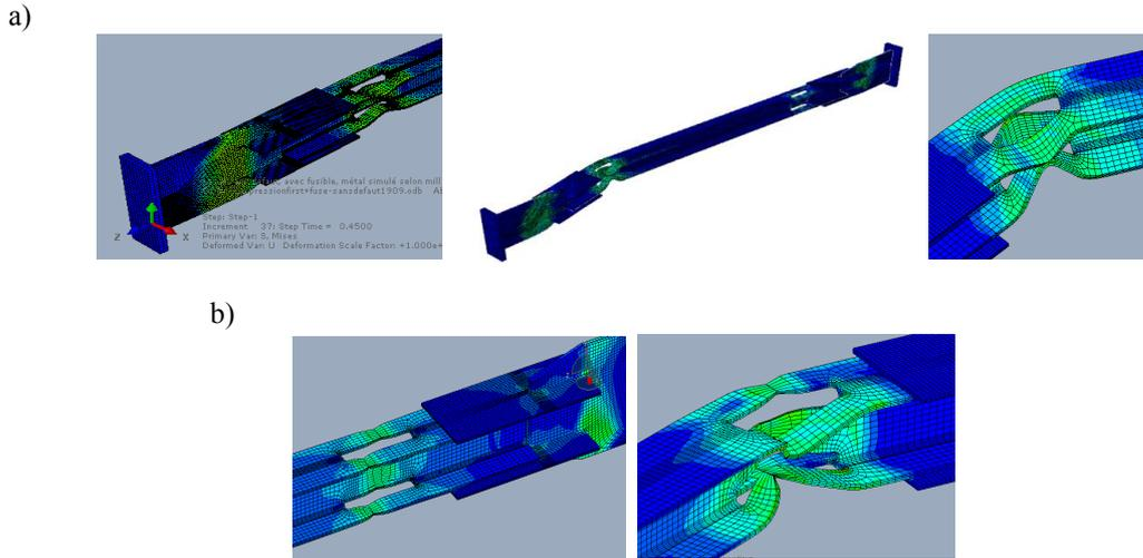
**Figure 3.** Inelastic response of the unconfined brace fuses: a) Local buckling response in the first compression excursion; b) Necking in tension (left) and buckling in compression (right) in the second cycle.
