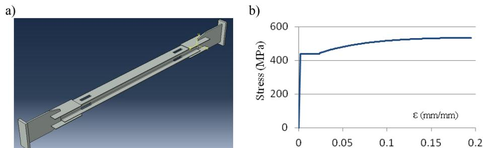
**Figure 2.** a) 3D Abaqus model of the brace; b) Steel properties from coupon test.
