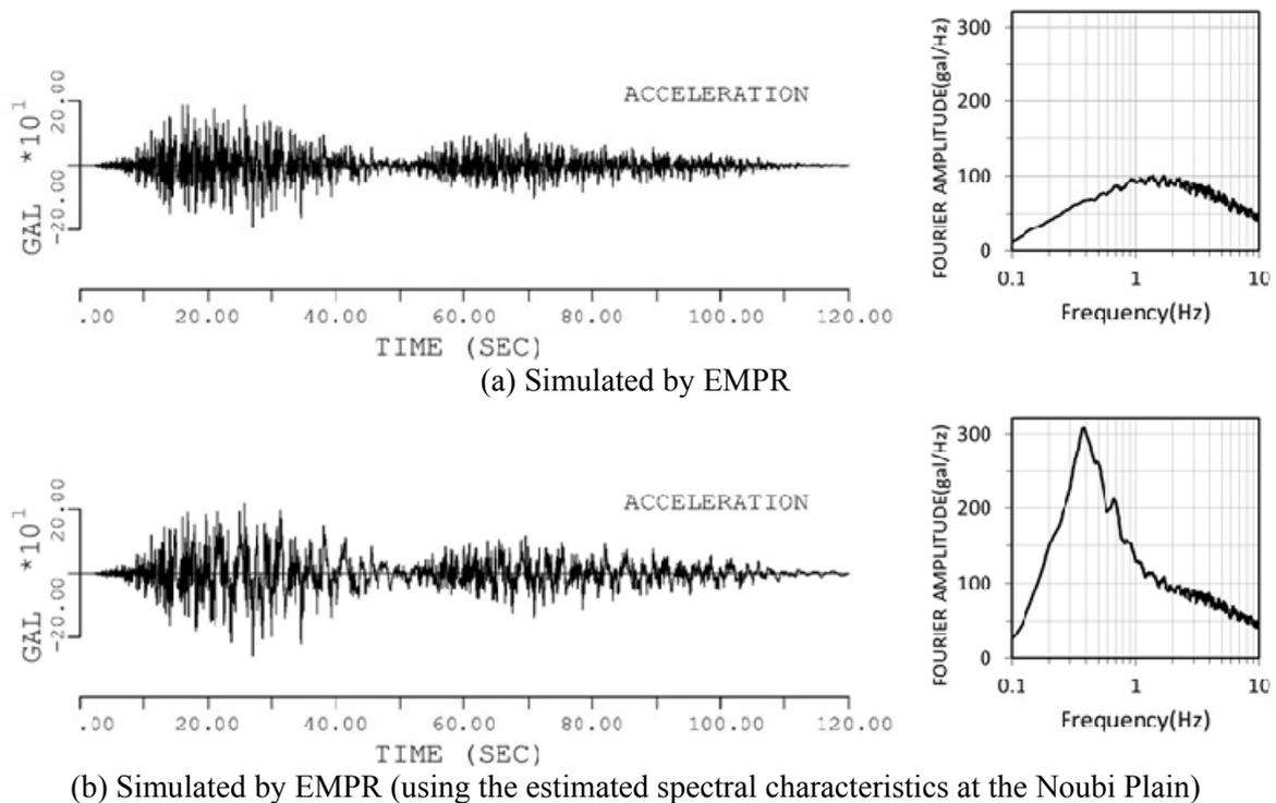
**Figure 4.5.** Comparison of acceleration time histories and fourier spectrum at the Port of Nagoya
