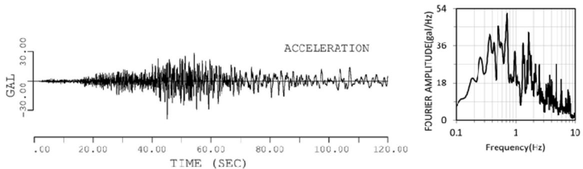
**Figure 4.6.** Recorded fourier spectrum at the Port of Nagoya (The off the Tokaido earthquake, EW)
