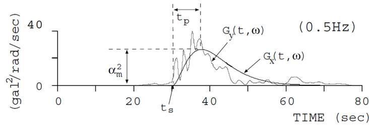
**Figure 2.1.** Recorded and simulated evolutionary power spectra
