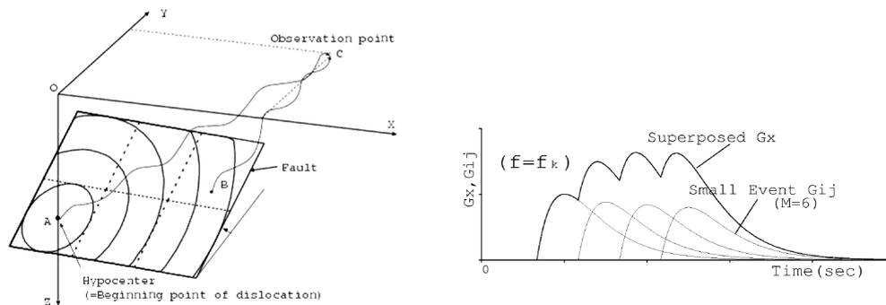
**Figure 2.2.** Fault modeling with multiple fault rupture and superposed evolutionary power spectra
