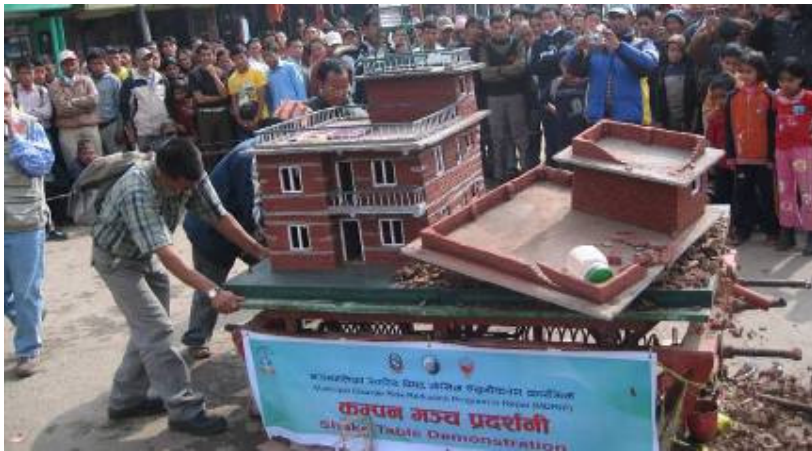
Figure 2. Observers check the endurance limit of an earthquake Resistant Model. The Earthquake Resistant Building was not damaged when the ordinary one collapsed when tested on the Shake Table / MDRIP.
