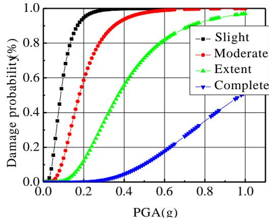
**Figure 3.3.** Model 2 seismic vulnerability curve
