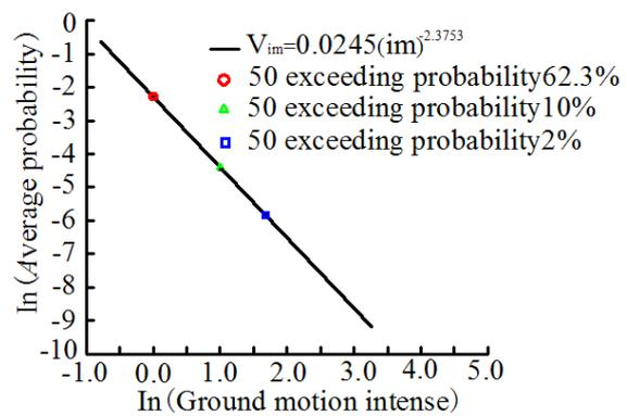
**Figure 1.2.** Linearized seismic hazard curve
