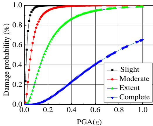
**Figure 3.4.** Model 3 seismic vulnerability curve
