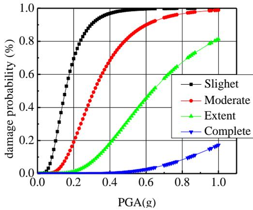
**Figure 3.2.** Model 1 seismic vulnerability curve
