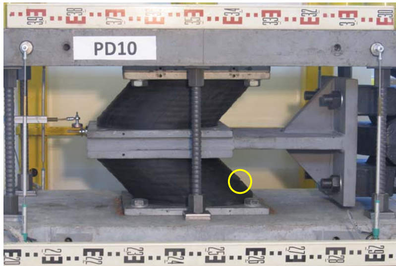
Figure 8. Deformed bearings at failure – note the damage in the yellow circle (PsD test PD10)
