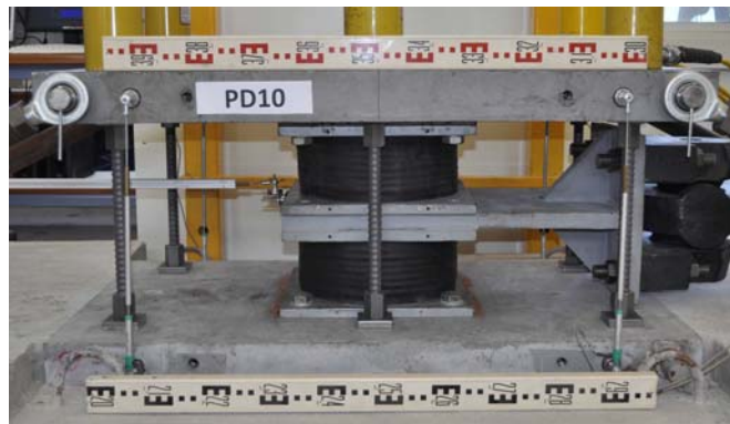
Figure 2. Photo of a pair of elastomeric bearings in parallel testing configuration
