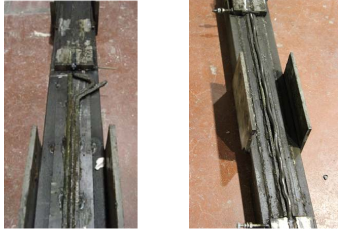
a) Rupture of the welding rod guide in MW4 b) Instability of the rod damper in test MW5
