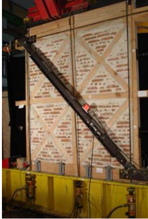
Figure 1. Walls MW4/5 with damper
