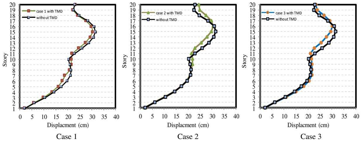
Figure 5.1. Comparing maximum lateral displacement in three cases.
