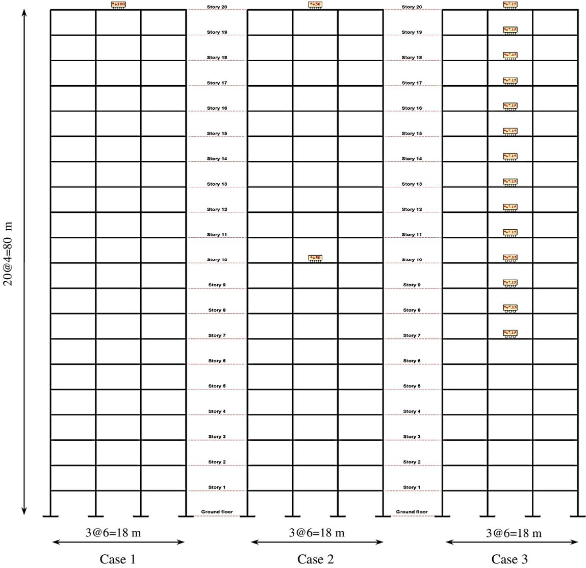
**Figure 4.1.** Twenty-story moment resistance frame showing location of TMDs
