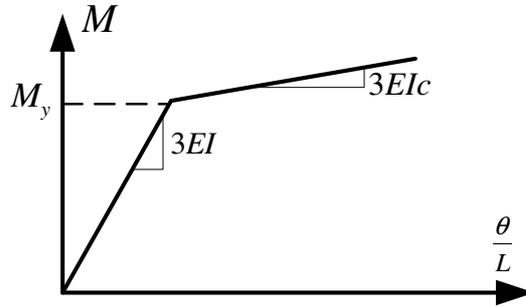
**Figure 3.2.** Relationship between member-end moment and chord angle before and after yielding.
