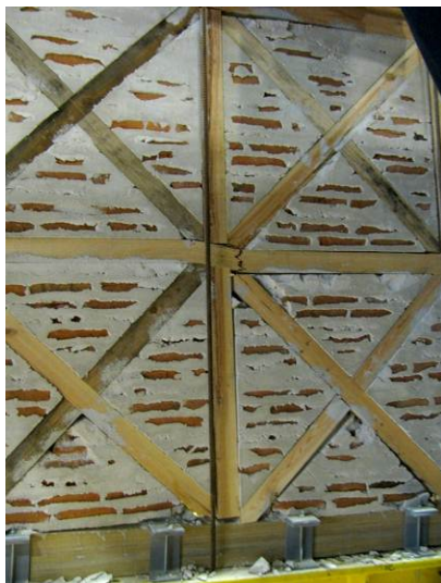
a) Failure by shear failure of intermediate timber beam for MW1
