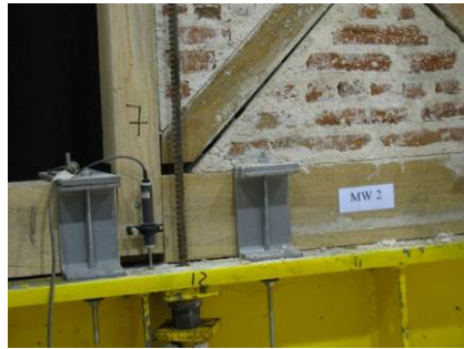
Figure 12. Vertical lift of bottom beam and vertical member.
