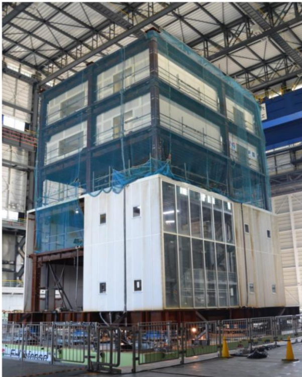
Figure 1. 5-story steel moment frame specimen set on triple pendulum isolators
