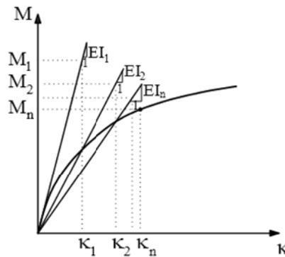
**Figure 3.1.** Secant stiffness method
