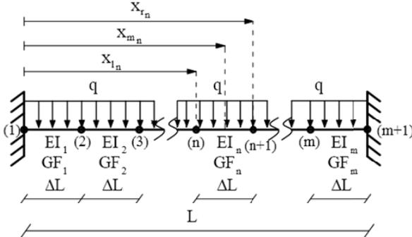
**Figure 2.2.** Meshed base element
