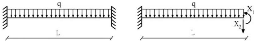
**Figure 2.1.** Beam-Column Element and the flexibility terms
