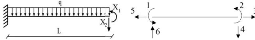
**Figure 2.5.** The degree of freedom of local axis system
