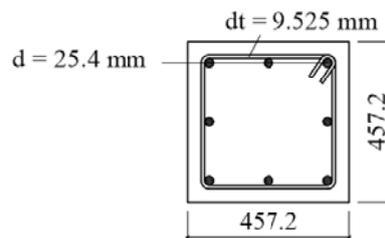
**Figure 4.1.** The cross section of flexure-shear critical specimen
