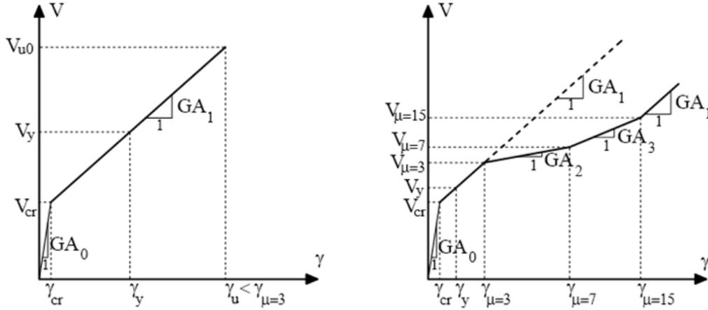
**Figure 3.2.** Shear distortion-shear force envelopes
