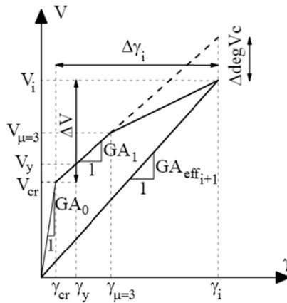
**Figure 3.4.** Implementation of shear-flexure interaction
