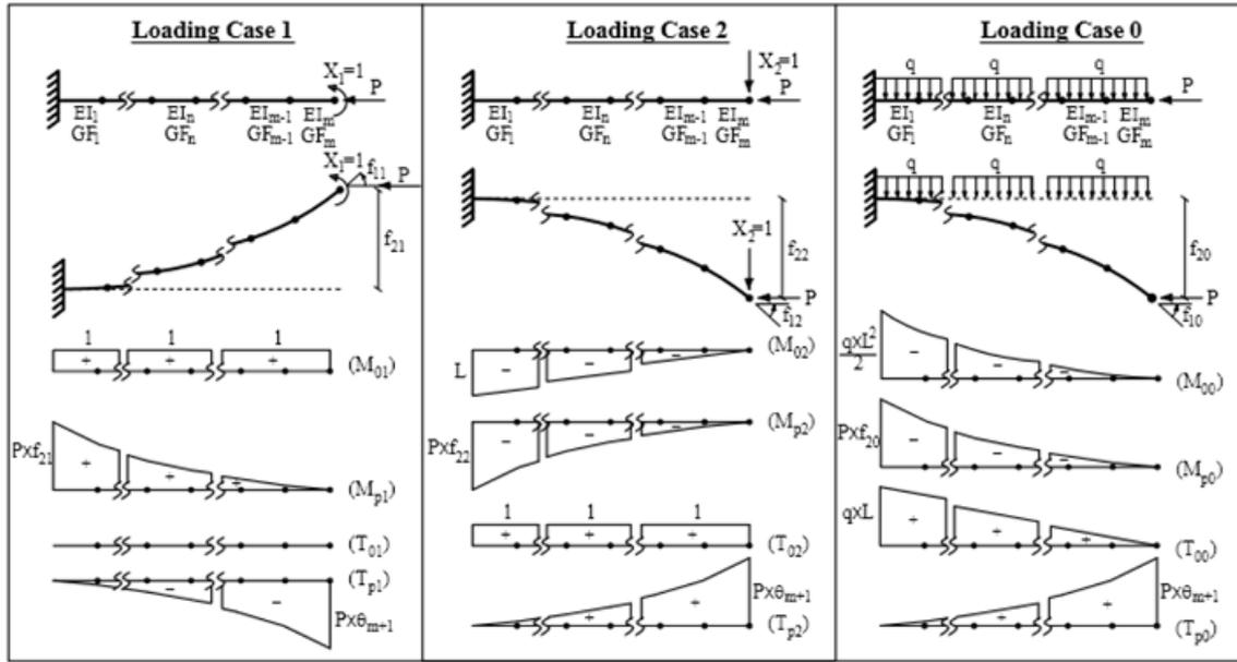
**Figure 2.4.** Moment and shear diagrams for different loading cases
