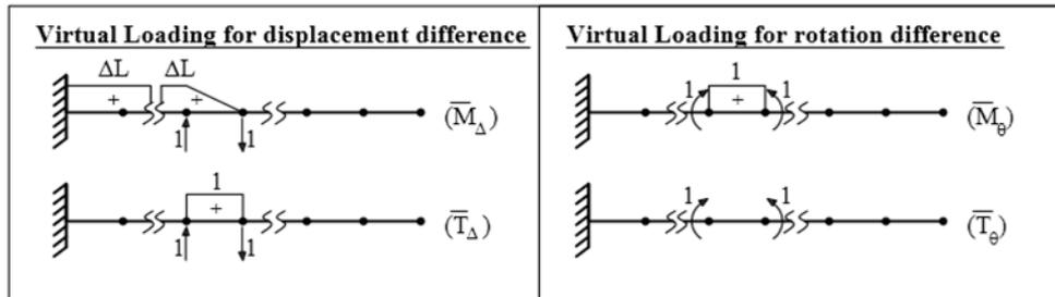
**Figure 2.3.** Virtual force and moment-shear diagrams for calculating rotation and displacement differences
