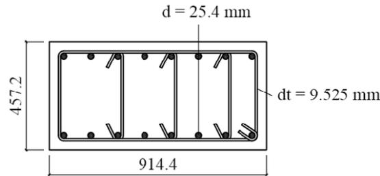
**Figure 4.3.** The cross section of shear critical specimen
