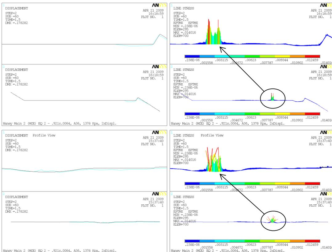
**Figure 10.** Typical Results from ANSYS Soil-Pipe Interaction Analyses for HM2 (10,000-yr Demand)
