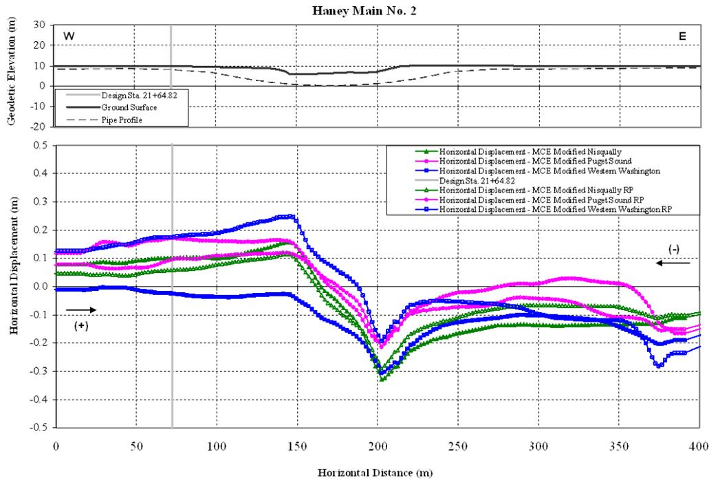
**Figure 9.** Computed Variations in Horizontal Displacement Profiles for HM2 (10,000-yr Demand)
