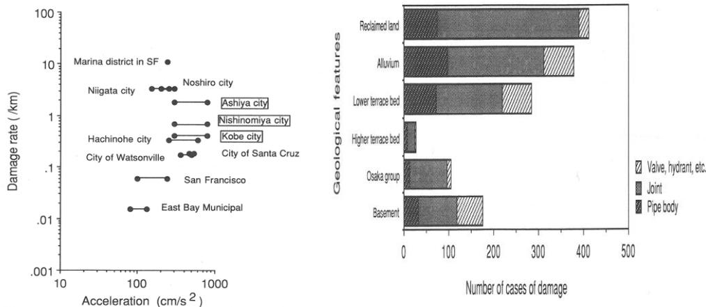
**Figure 2.** Pipeline Damage Statistics for Water Mains -Past Earthquakes (After Kitaura and Miyajima)
