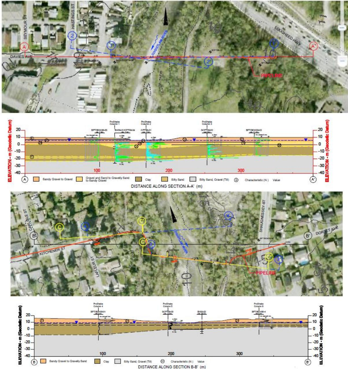
Figure 4. Plan Location and Soil Stratigraphy at HM3
