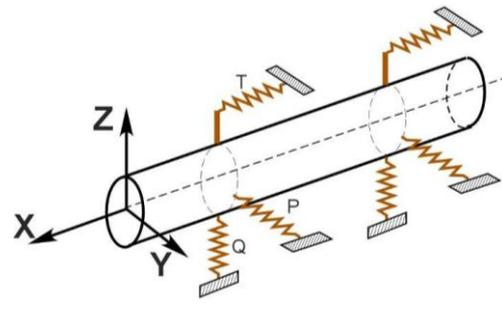
**Figure 6.** Soil Restraint to Pipe Movement Modelled Using 3D Non-Linear Springs
