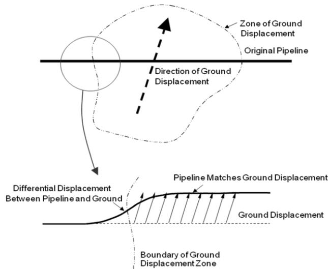
**Figure 5.** Pipeline Response to Ground Movements
