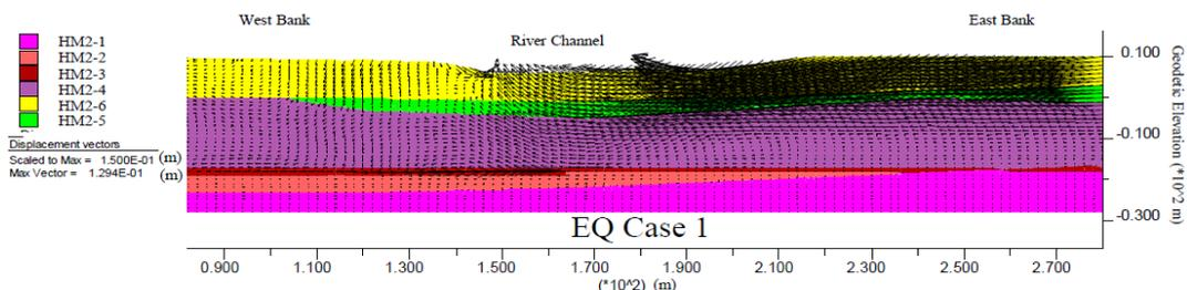
**Figure 8.** Typical Ground Displacement Patterns Computed for HM2 (2,475-yr Demand)
