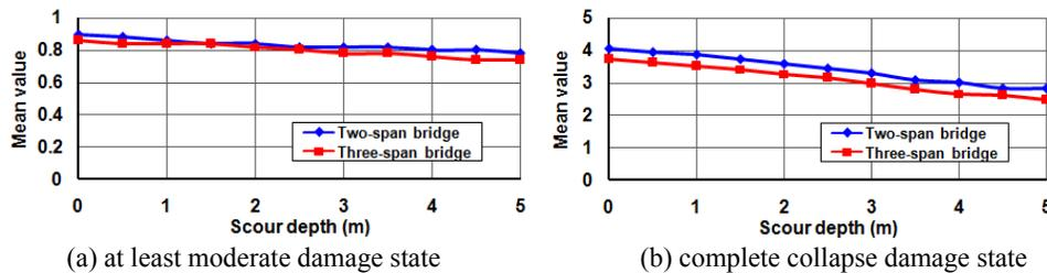
**Figure 6.** Change in the mean values of seismic fragility curves by scour depth
