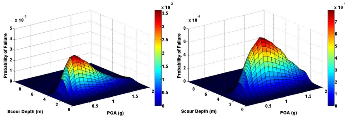
**Figure 8.** Joint probability of failure of two-span bridges at moderate damage state (left) and major damage state (right)
