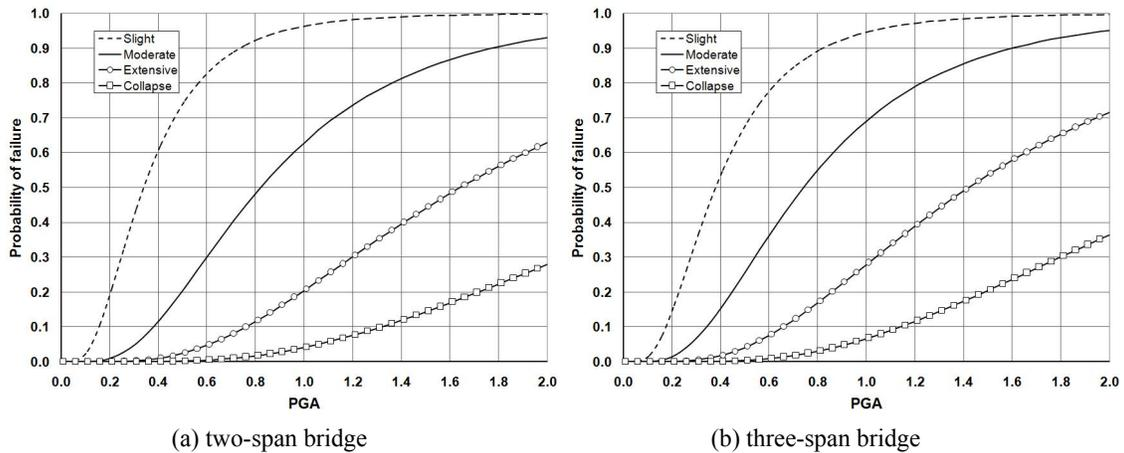
**Figure 5.** Developed fragility curves for the case study bridges without any scouring effects
