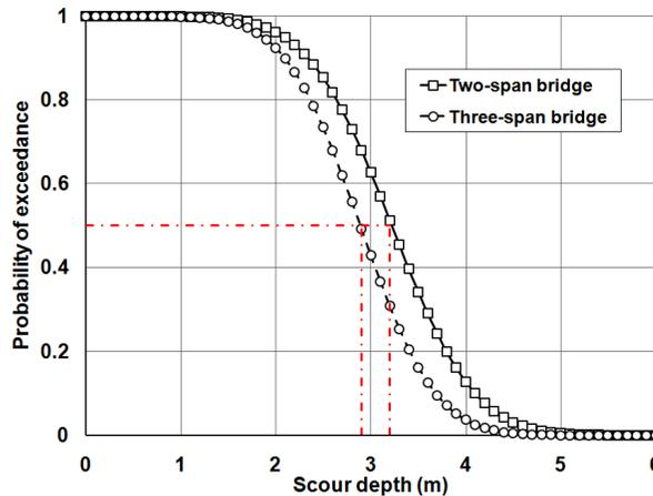
**Figure 3.** Developed risk curves for the two- and three-span bridges under different scour depths
