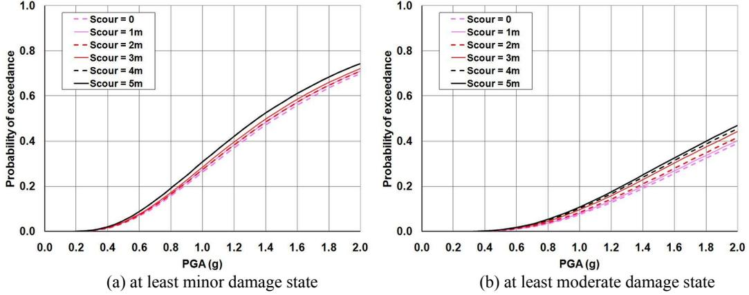
**Figure 7.** Developed fragility curves for the three-span bridge with different scour depths
