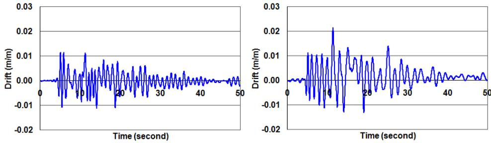
**Figure 4.** Time-history of deck drift ratio for the two-span bridge at the scour depth of 0.5m (left) and 5.0m (right)
