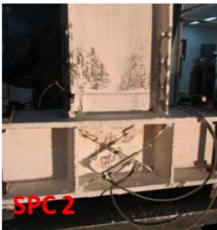
Figure 4.2. Formation of plastic hinge in the beam and panel zone of the second sample
