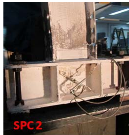
Figure 4.3. Method of rupture in the second sample
