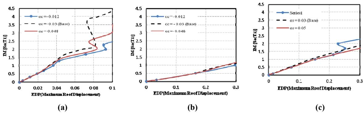
Figure 10. Sensitivity of Maximum Roof Displacement to  $\alpha_c$ : a) FM03B1, b) FM07B1 and c) FM12B3
