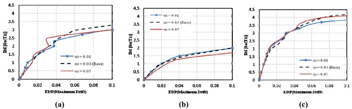
Figure 8. Sensitivity of Maximum Interstory Drift to  $\alpha_s$ : a) FM03B1, b) FM07B1 and c) FM12B3.
