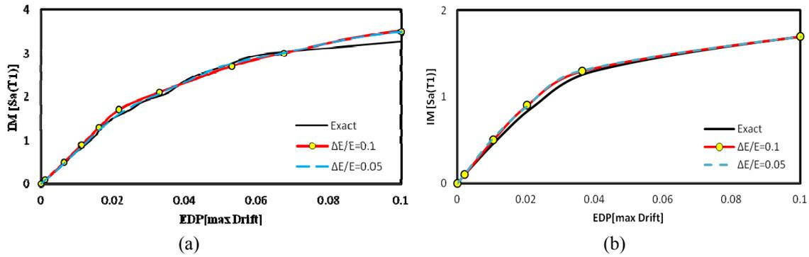
**Figure 5.** Sensitivity of Maximum Interstory Drift ratio to modulus of elasticity: a) FM03B1, b) FM07B1
