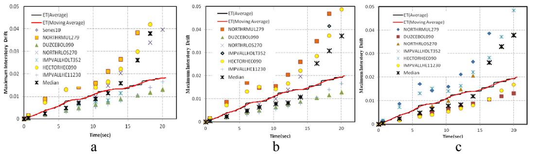
Figure 16. Maximum Interstory Drift Consider of changing  $\delta_c/\delta_y$ : a) FM03B1, b) FM07B1 and c) FM12B3.
