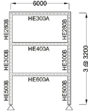
**Figure 1.** Schematic representation of the 3-story 1-bay
