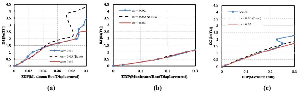
Figure 11. Sensitivity of Maximum Roof Displacement to  $\alpha_s$ : a) FM03B1, b) FM07B1 and c) FM12B3
