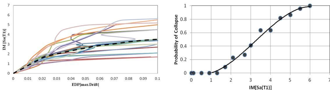
**Figure 3.** Collapse fragility curve using IDAs-FM03B1: a) IM-EDP plot, b) Collapse fragility curve
