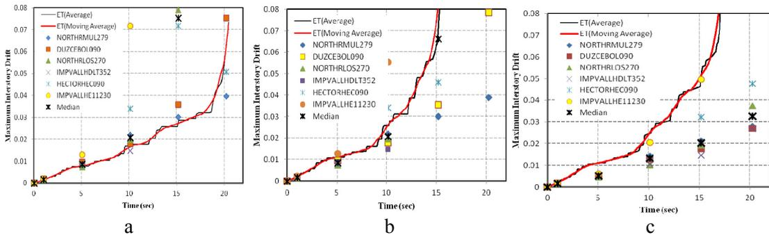
Figure 15. Maximum Interstory Drift Consider of changing  $\alpha_s$ : a) FM03B1, b) FM07B1 and c) FM12B3.
