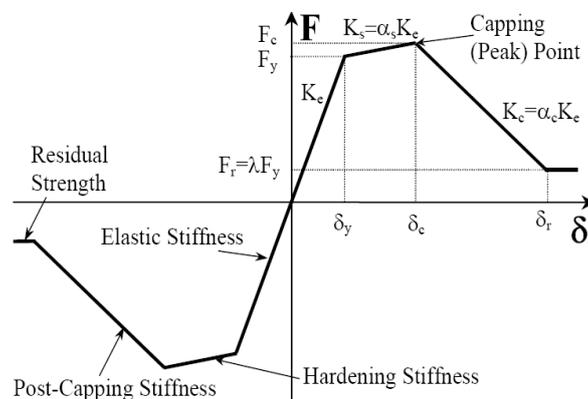
**Figure 2.** Necessary parameters for defining the SSD model (Ibarra and Krawinkler, 2005).
