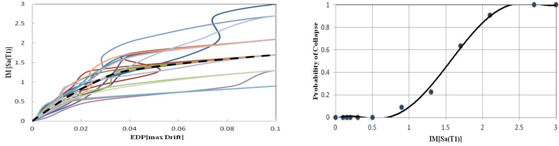
**Figure 4.** Collapse fragility curve using IDAs-FM07B1: a) IM-EDP plot, b) Collapse fragility curve
