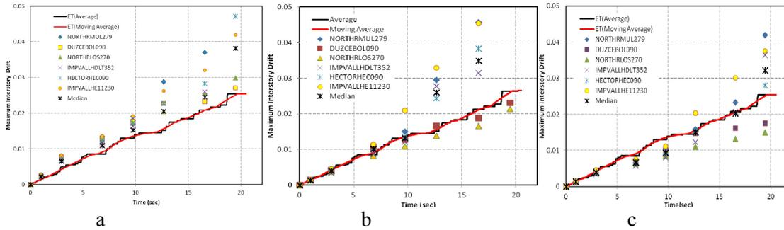
Figure 14. Maximum Interstory Drift Consider of changing  $\alpha_c$ : a) FM03B1, b) FM07B1 and c) FM12B3.
