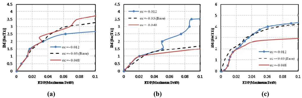
Figure 7. Sensitivity of Maximum Interstory Drift to  $\alpha_c$ : a) FM03B1, b) FM07B1 and c) FM12B3.
