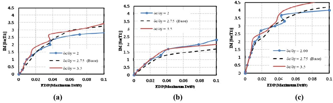
Figure 9. Sensitivity of Maximum Interstory Drift to  $\delta c/\delta y$ : a) FM03B1, b) FM07B1 and c) FM12B3.
