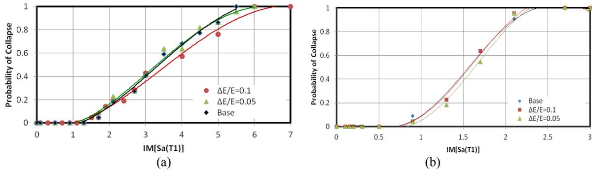
**Figure 6.** Sensitivity of Collapse fragility Curve to modulus of elasticity: a) FM03B1, b) FM07B1
