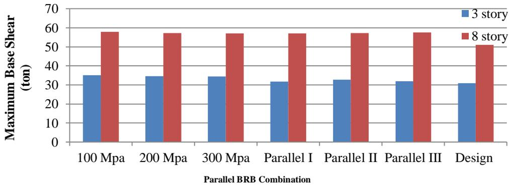
Fig. 4.5. Variation of maximum base shear for 3 and 8 story structures for 6 different parallel BRB combinations.
