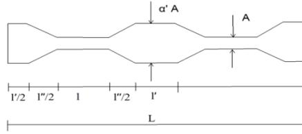
**Figure 2.1** different components of two BRBs in series
