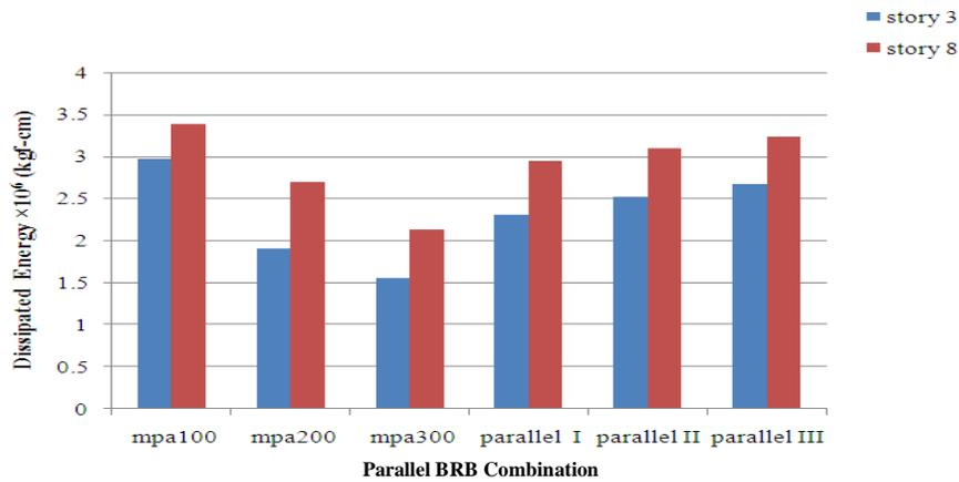
**Fig. 4.2.** Variation of dissipated energy for 3 and 8 story structures with 6 different parallel BRB combinations
