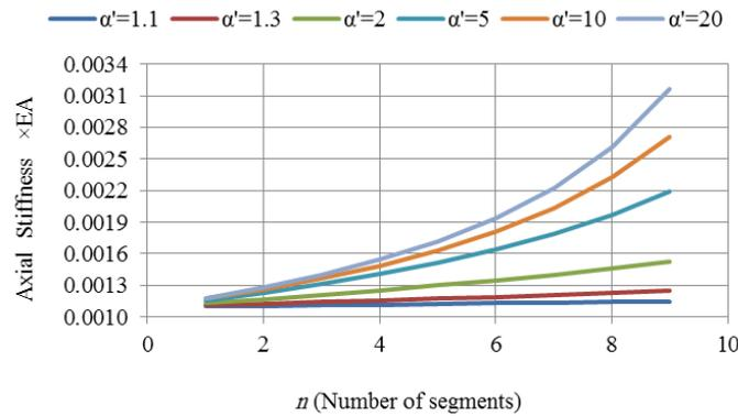
**Figure 2.3** Variation of equivalent stiffness of  $n$  equal BRBs in series, for different area ratios,  $\alpha'$ .
