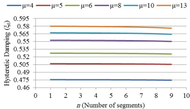
**Figure 2.7.** Variation of hysteretic damping,  $\zeta_o$ , of  $n$  equal BRBs in series for different values of ductility ratio,  $\mu$ .
