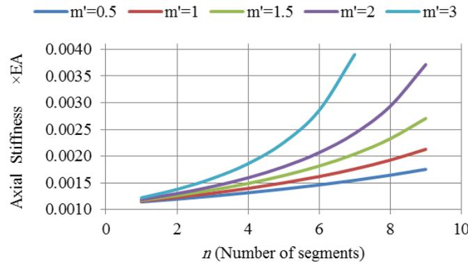
**Figure 2.2** Variation of equivalent stiffness of  $n$  equal BRBs in series, for different  $m'$  ratios.
