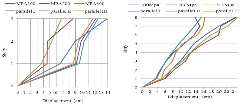
Fig. 4.4. Variation of story displacement along the height for 3 and 8 story structures for 6 different parallel BRB combinations
