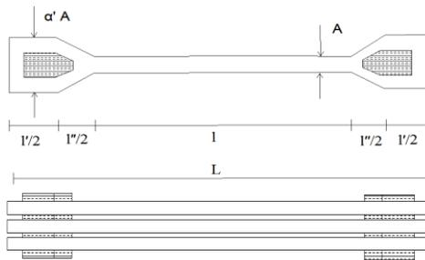
**Figure 3.1.** Geometric properties of a typical three segmented parallel BRB.
