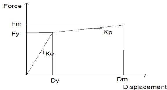
**Figure 2.4.** Bilinear force-displacement relationship  $n$  equal BRBs in series.
