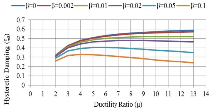
**Figure 2.6.** Variation of hysteretic damping,  $\zeta_o$  serial-equal BRBs with ductility ratio,  $\mu$  for different  $\beta$  ratios.
