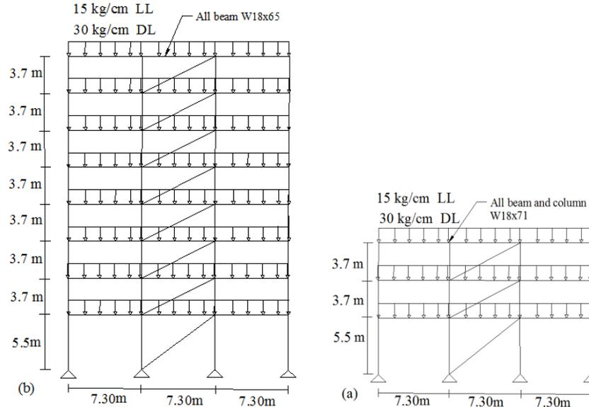
**Fig. 4.1.** 3 and 8 story model structures with 6 different parallel BRB combinations.
