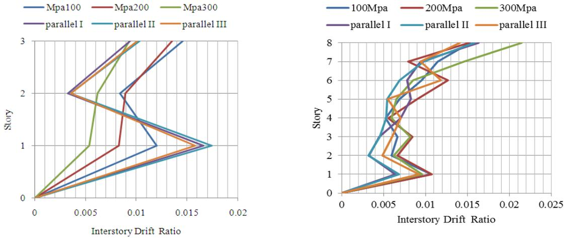
Fig. 4.3. Variation of interstory drift ratio along the height for 3 and 8 story structures for 6 different parallel BRB combinations
