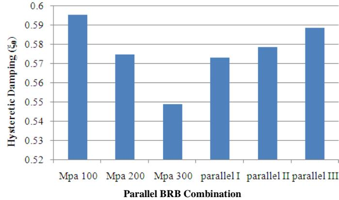
**Figure 3.3.** Variation of hysteretic damping,  $\xi_0$  for different combination of BRBs in parallel
