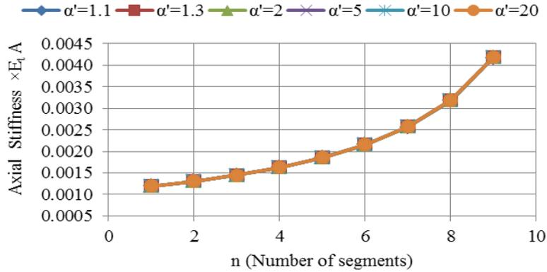
**Figure 2.5.** Variation of equivalent post-yield stiffness  $n$  equal BRBs in series, for different area ratios,  $\alpha'$ .
