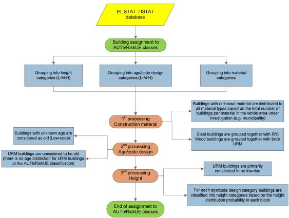
Figure 2.1. Flowchart of the building classification 'algorithm'
