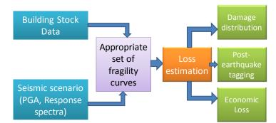
Figure 5.1. The AUTh/ EPPO-ITSAK loss estimation procedure scheme
