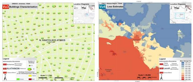
Figure 4.2. Predicted distribution of post-earthquake damage distribution in terms of green-yellow-red tagging for Athens (left) and Mean Damage Factor for L'Aquila (right)
