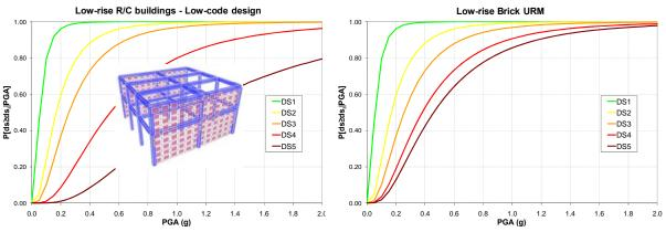
Figure 3.1. Fragility curves in terms of PGA for low code, low rise with frame system (left) and low rise, brick URM buildings (right)
