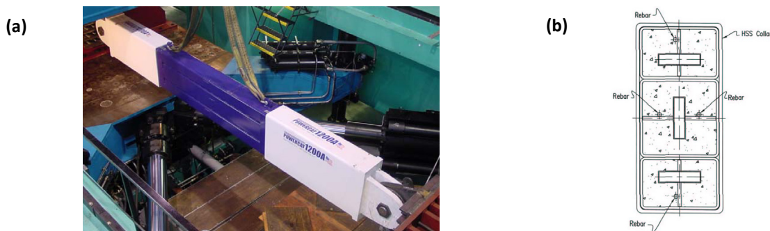
Figure 2.3. Multi core BRB (Merritt et al. 2003), (a) Overview (b) Cross sectional view
