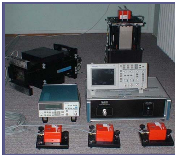
Figure 4. Accelerometers for the building screening
