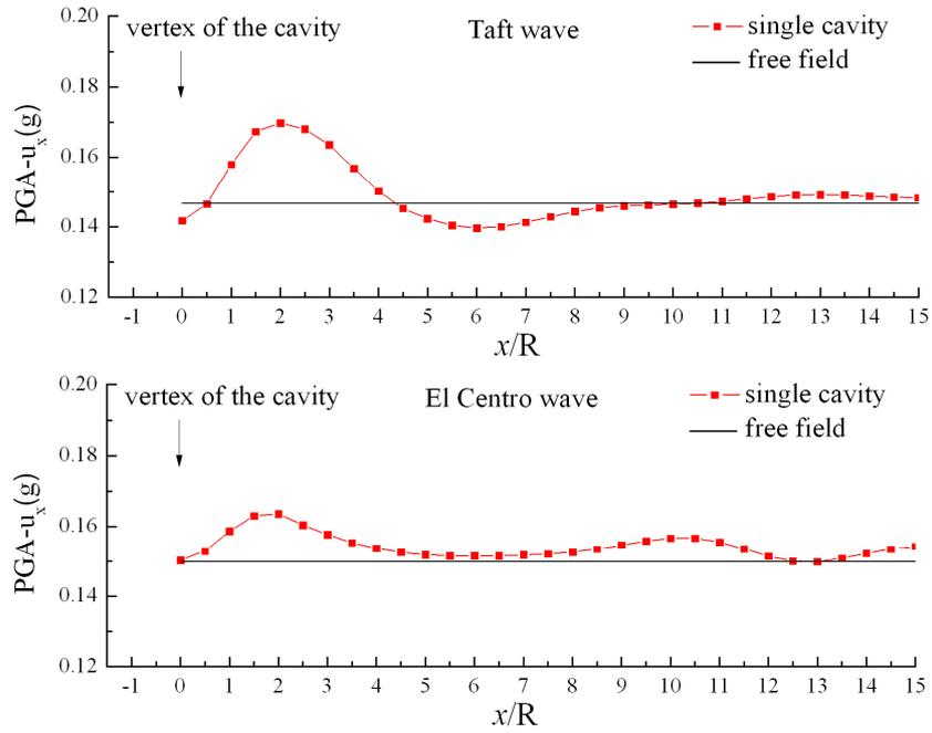
**Figure 3.** Envelope of horizontal PGAs at surface of half-space with single cavity
