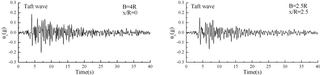
**Figure 11.** Horizontal acceleration time histories with twin cavities for incident Taft wave
