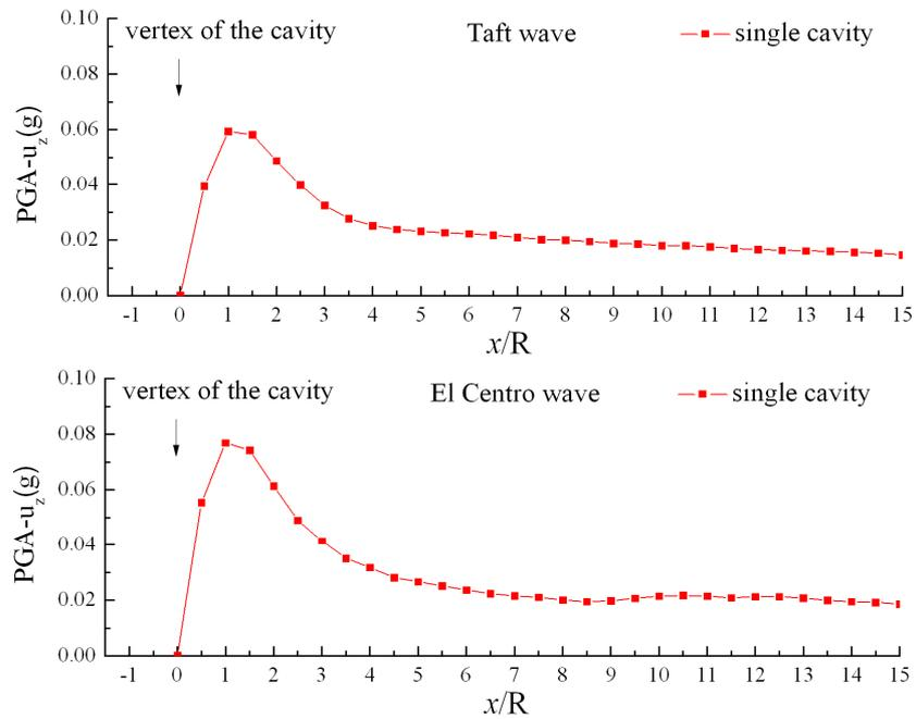
**Figure 4.** Envelope of vertical PGAs at surface of half-space with single cavity
