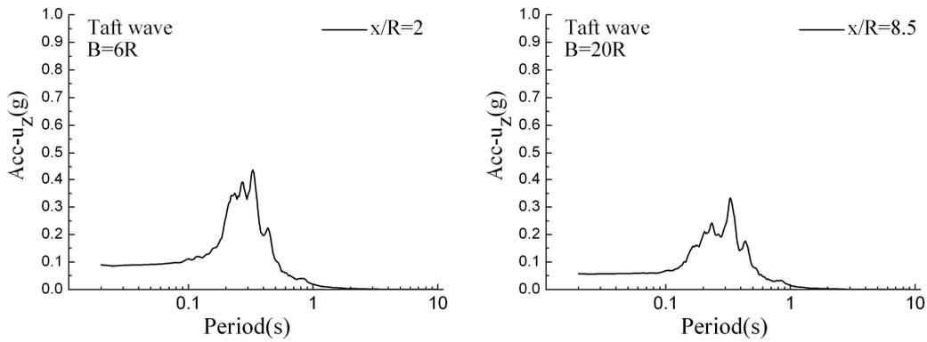
**Figure 16.** Vertical response spectrum with twin cavities for incident Taft wave
