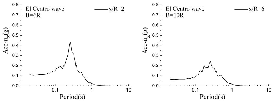
**Figure 18.** Vertical response spectrum with twin cavities for incident El Centro wave
