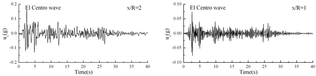
**Figure 6.** Surface acceleration time histories with single cavity for incident El Centro wave
