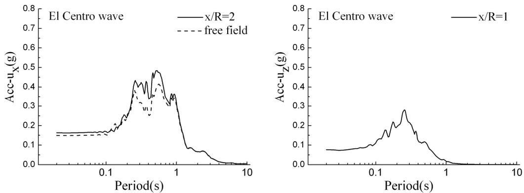
**Figure 8.** Acceleration response spectrum with single cavity for incident El Centro wave
