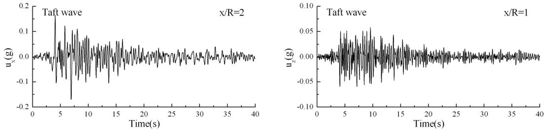
**Figure 5.** Surface acceleration time histories with single cavity for incident Taft wave
