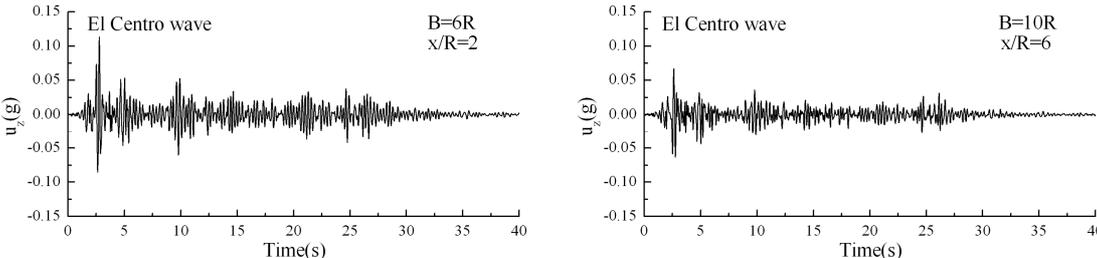
**Figure 14.** Vertical acceleration time histories with twin cavities for incident El Centro wave
