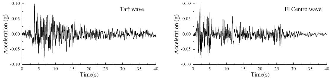
**Figure 2.** Incident seismic waves
