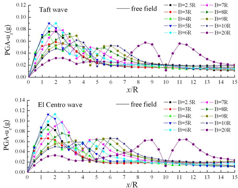
**Figure 10.** Envelope of vertical PGAs at surface of half-space with twin cavities
