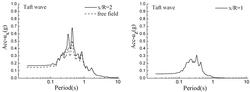
**Figure 7.** Acceleration response spectrum with single cavity for incident Taft wave
