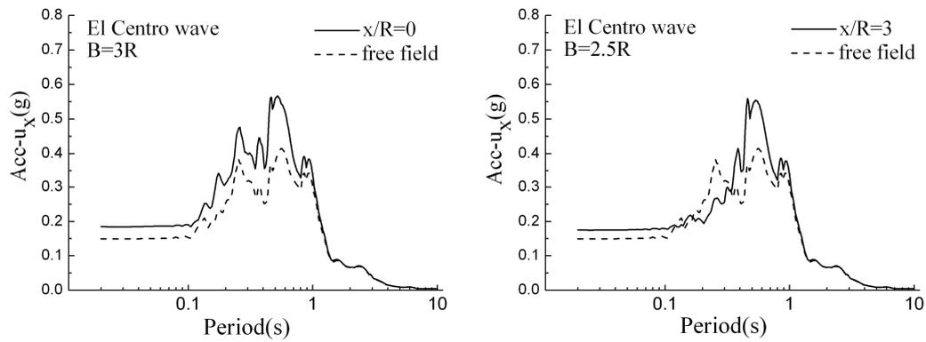
**Figure 17.** Horizontal response spectrum with twin cavities for incident El Centro wave
