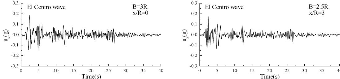
**Figure 13.** Horizontal acceleration time histories with twin cavities for incident El Centro wave
