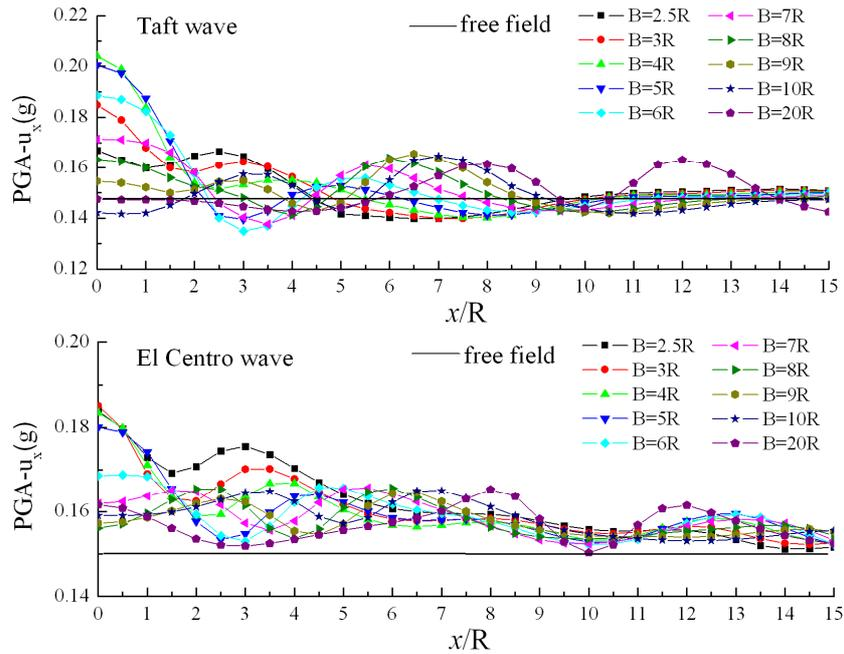
**Figure 9.** Envelope of horizontal PGAs at surface of half-space with twin cavities
