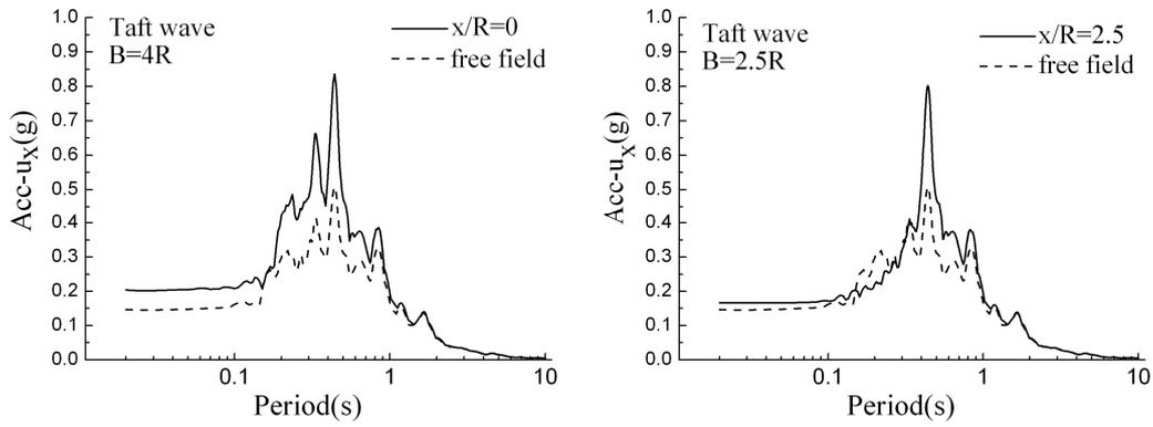
**Figure 15.** Horizontal response spectrum with twin cavities for incident Taft wave
