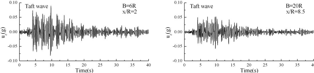
**Figure 12.** Vertical acceleration time histories with twin cavities for incident Taft wave
