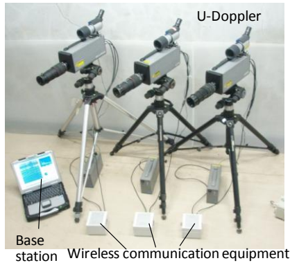
Figure 8. 3D remote vibration measurement system
