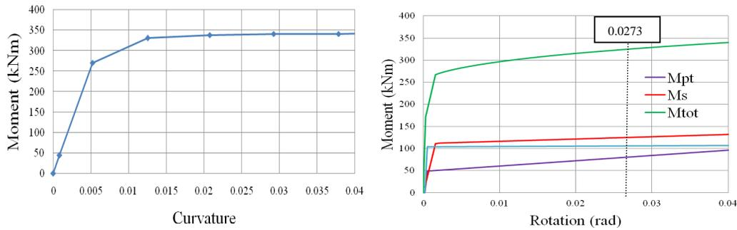
**Figure 3.3.** Moment-curvature, monolithic section (left); equivalent DCR section (right)
