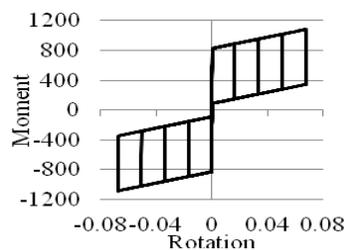
**Figure 3.9.** Multi pier model with friction dissipators
