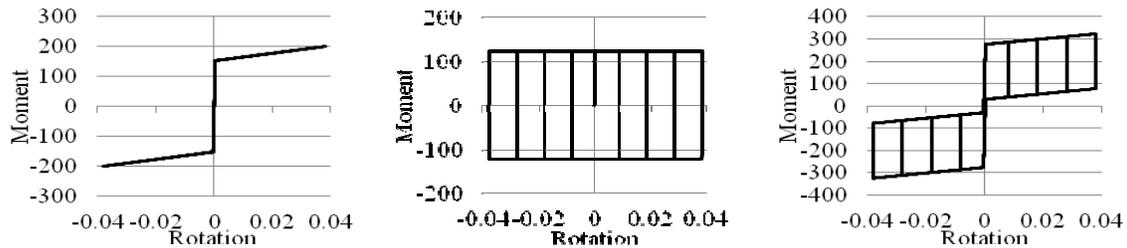
**Figure 3.7.** Single pier with friction dissipators; self-centering (left); dissipator (middle); total hysteresis (right)
