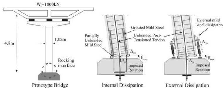
**Figure 2.3.** DCR concept with internal and external dissipation devices (Marriott, 2009)
