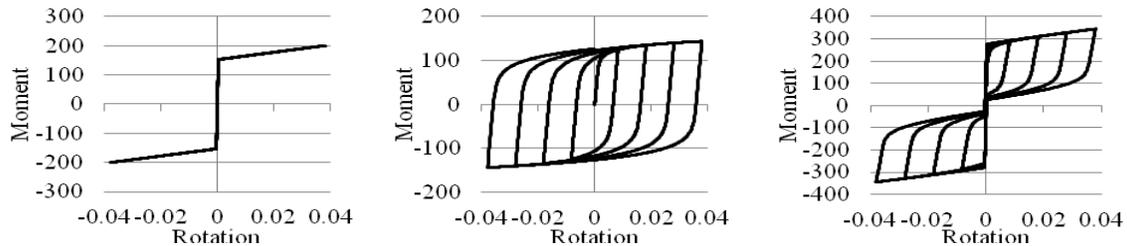
**Figure 3.6.** Single pier with yielding dissipators; self-centering (left); dissipator (middle); total hysteresis (right)
