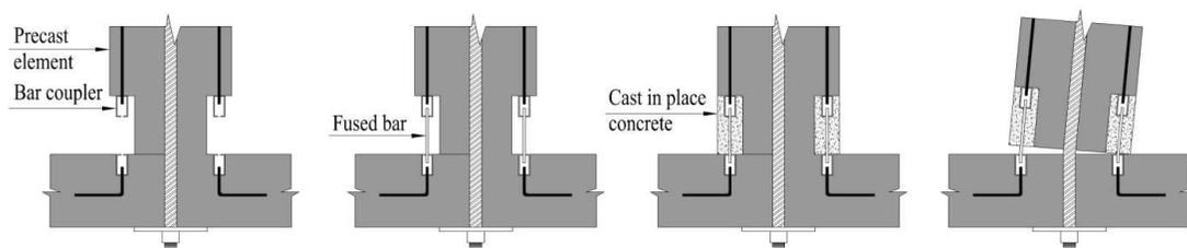
**Figure 3.5.** Construction sequence and activation mechanism of the internal bar system
