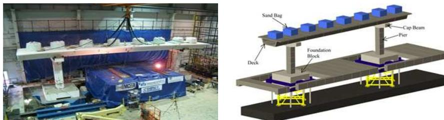
**Figure 2.2.** Half-scale post-tensioned segmented bridge system (Sideris et al 2010)
