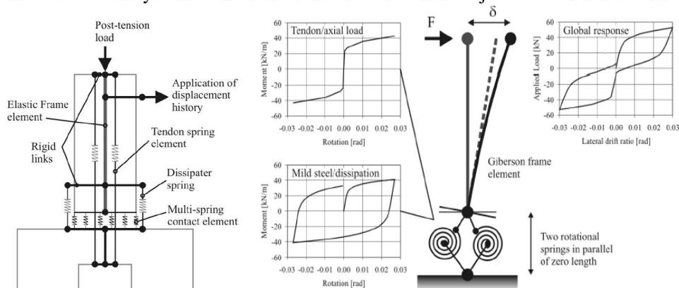
**Figure 2.5.** Multi-spring model (left); lumped plasticity model (right), (Marriot, 2009)
