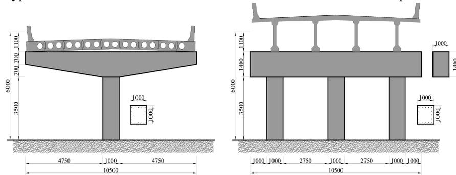
**Figure 3.1.** Prototype A (single pier support) (left); Prototype B (multi pier support) (right)
