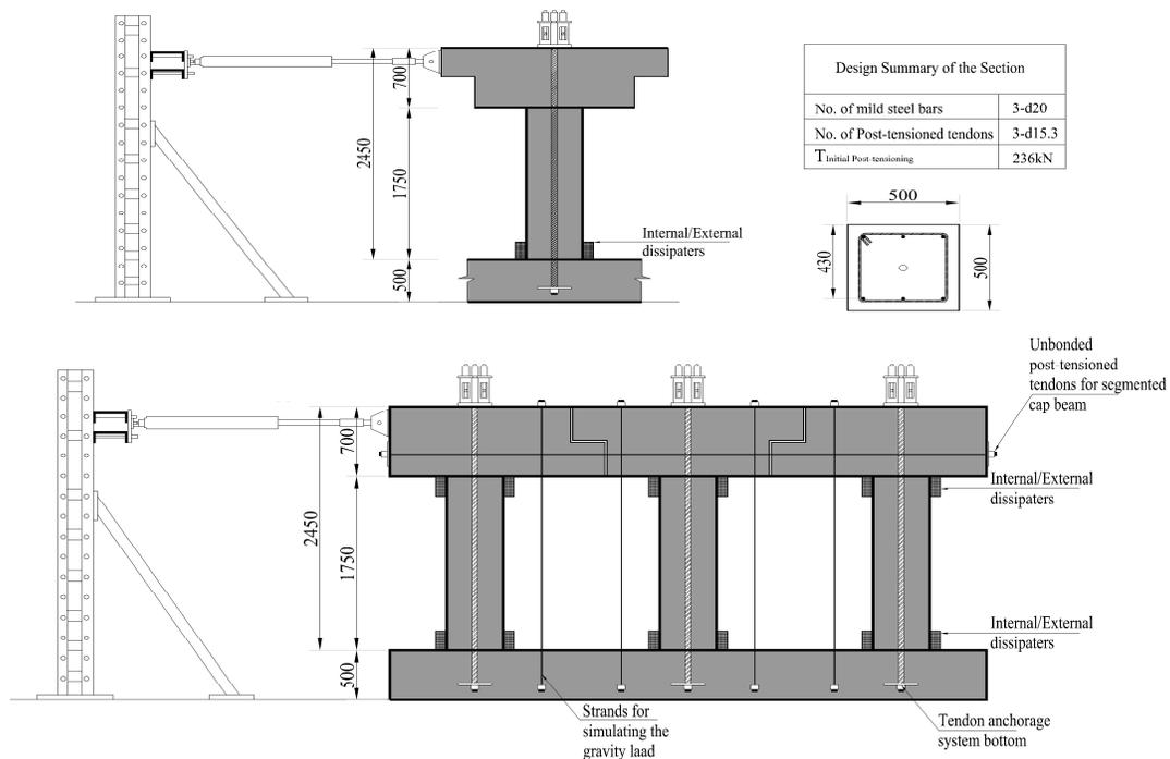
**Figure 3.2.** Experimental test setup, single pier (top); multi pier (bottom)
