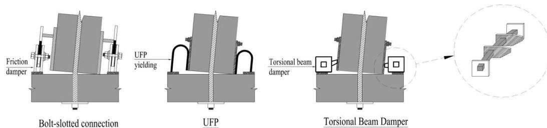
**Figure 3.4.** Activation mechanisms for each dissipator at the rocking interface
