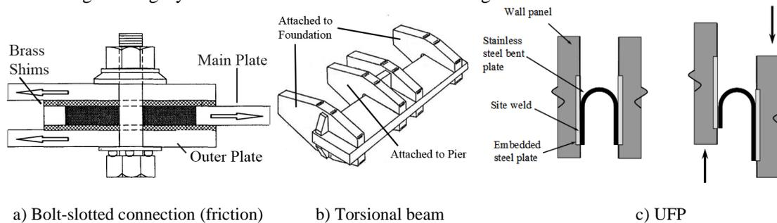
**Figure 2.4.** Examples of external dissipators
