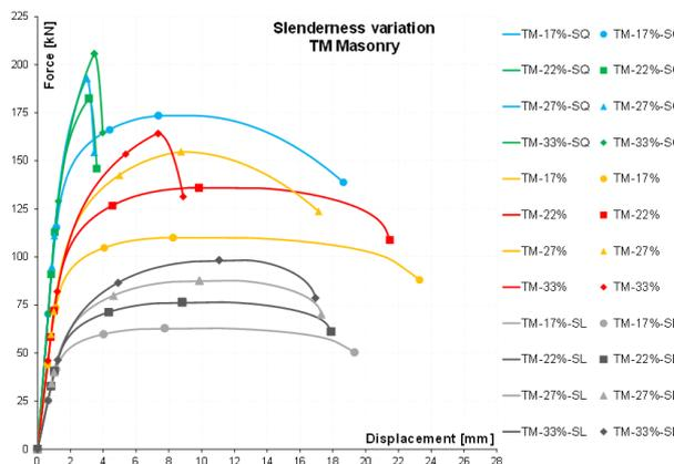
**Figure 5.** URM Parametric shear-compression analyses. Variation of slenderness ratio.
