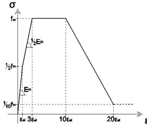
Figure 3. Masonry stress-strain relation.
