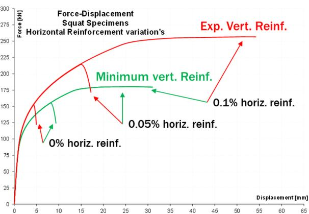
**Figure 6.** RM Parametric shear-compression analyses. Variation of horizontal reinforcement ratio. Case of squat walls with  $\sigma_0=0.6$  N/mm<sup>2</sup>
