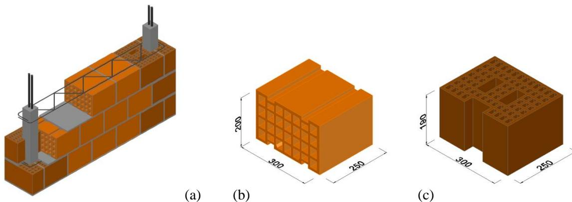
**Figure 2.** (a) Reinforced Masonry system (RM); (b) horizontally perforated unit and (c) vertically perforated unit.
