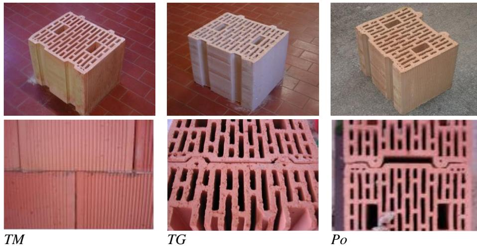
**Figure 1.** The three unreinforced masonry unit types: TM TG and Po.
