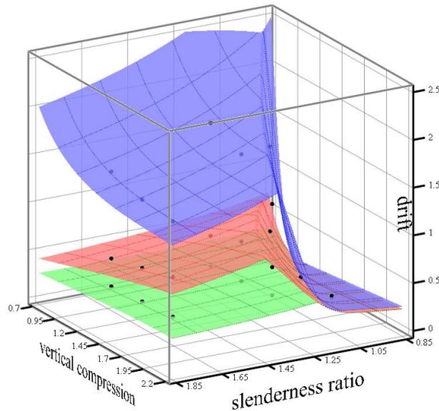
**Figure 8.** Graphical view of different drift limit-states (black dots) for slenderness variation (TM masonry). Surfaces deriving from EQ: maximum drift (blue), drift at  $F_{max}$  (red) and critical drift (green).
