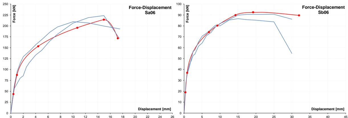
Figure 4. Model (red line) versus Experimental (blue lines) load-displacement capacity curves (the positive and negative displacement envelopes for  $\sigma_0=0.6$  N/mm<sup>2</sup>). Reinforced masonry H/L=1.09 (left) and H/L=1.63 (right).
