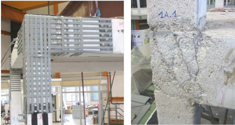
Figure 8. (a) View of joint 1A-2 during tests in Stage 2; and (b) joint 1A-1 after removing the PTMS
