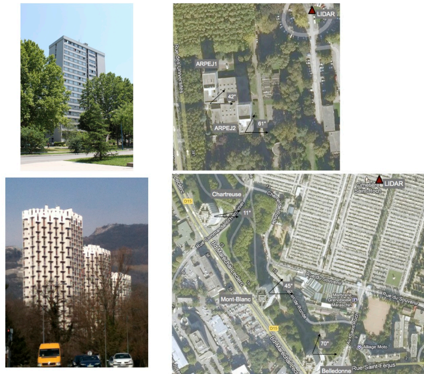
Figure 5: Description of the five buildings (ARPEJ1 and ARPEJ2, upper row - Ile Verte towers, lower row) tested by ambient vibrations and Lidar techniques. The red triangle corresponds to the position of the Lidar for recordings and the orientation of the buildings are provided by the black arrows.
