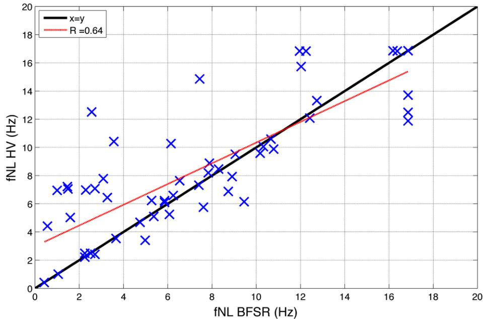
Figure 6. Correlation between fNL (calculate from linear to nonlinear ratio of BFSR or H/V) with  $f_0$  and  $f_{pred}$ .
