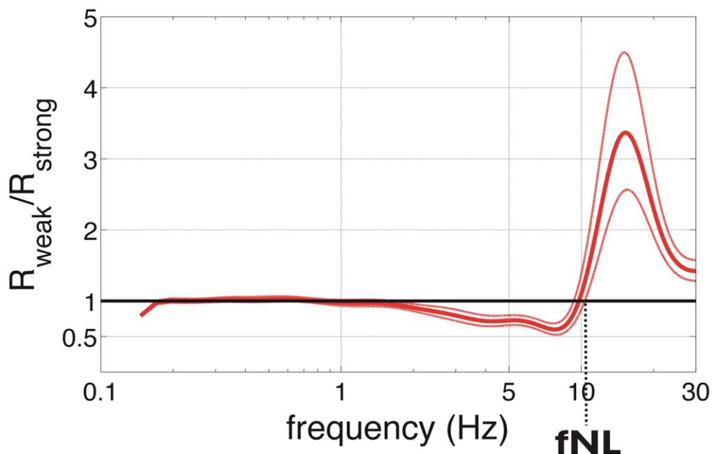
Figure 2. Ratio of site response computed from weak motion and strong motion (mean and 65% confidence limit) at IWTH23. The nonlinear parameter fNL represents the frequency from which this ratio is significantly above one (ie: lower band of the 65% confidence limit is above one).
