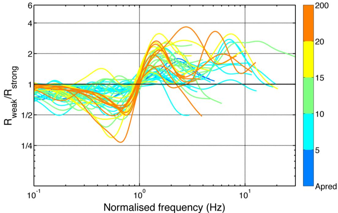
Figure 3. Ratio of the Borehole Fourier Spectral Ratio (BFSR) computed with weak motion and strong motion according to the maximum amplitude of the mean linear BFSR, the frequency is normalized by the FNL of each site.
