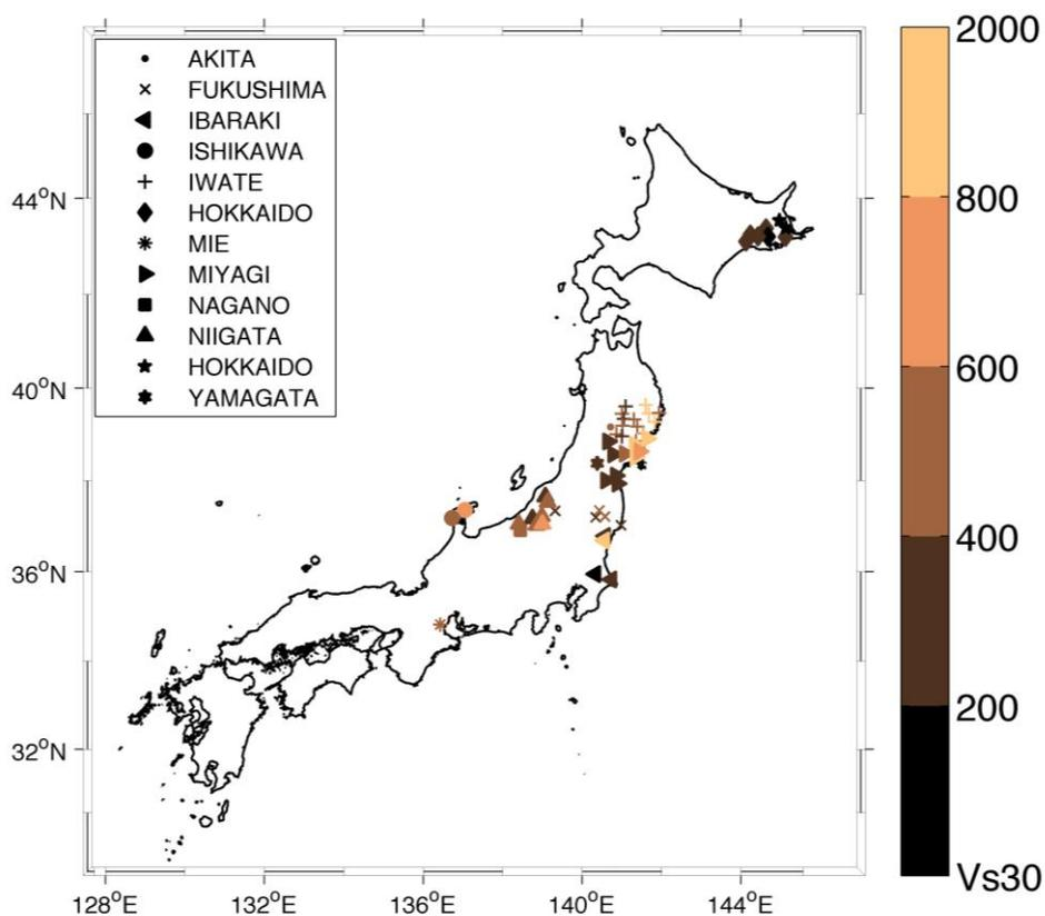
Figure 1. Location of the 54 KiK-net sites that have recorded at least two events with PGA at depth higher than  $50 \text{ cm/s}^2$ .
