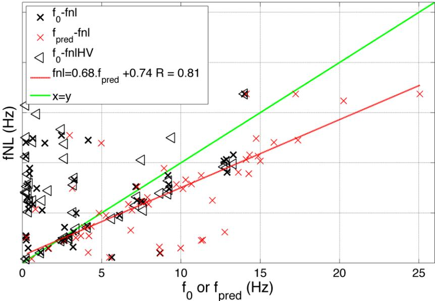
Figure 5. Correlation between fNL (calculate from linear to nonlinear ratio of BFSR or H/V) with  $f_0$  and  $f_{pred}$ .
