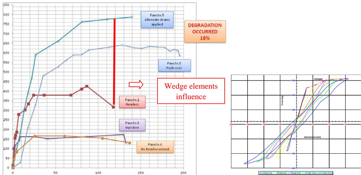
**Figure 3.3.** Panel n. 5 alternate directions test and panels' pushover final comparison
