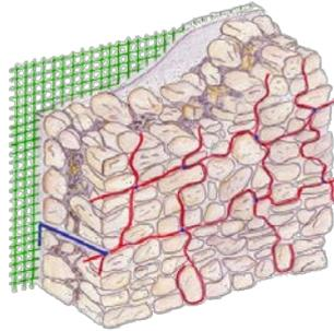
**Figure 2.3.** Panel n. 1 – reinforcement approach: Reticolatus(external surface) and GFRP reinforced plaster (internal surface).
