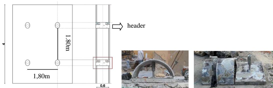
**Figure 2.6.** Panel n. 2 – Strengthening method: headers setting and abductor wedge provided.
