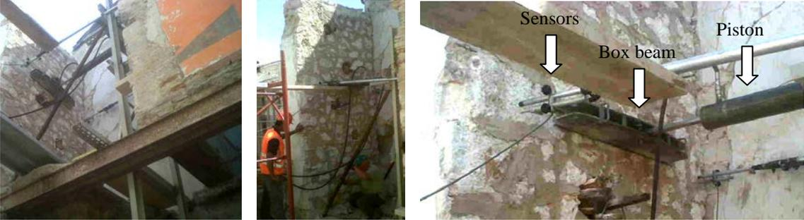
**Figure 3.2.** Panel n. 5 –Set-up details
