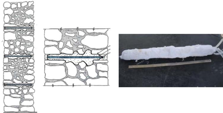
**Figure 2.8.** Panel n. 3 – Injection anchors with sock-like headers – schematic plan for irregular stonework (transversal section) and header photo after panel test.
