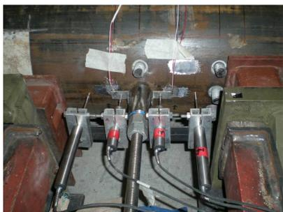
Figure 6. Test setup for CABBs anchorage test
