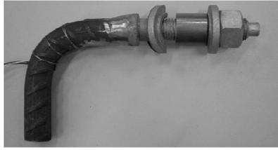
**Figure 1.** Cogged Anchored Blind Bolt (CABB)
