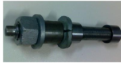
**Figure 2.** Headed Anchored Blind Bolt (HABB)
