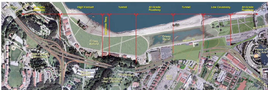
Figure 1.2. Alignment of future Presidio Parkway, San Francisco, CA
