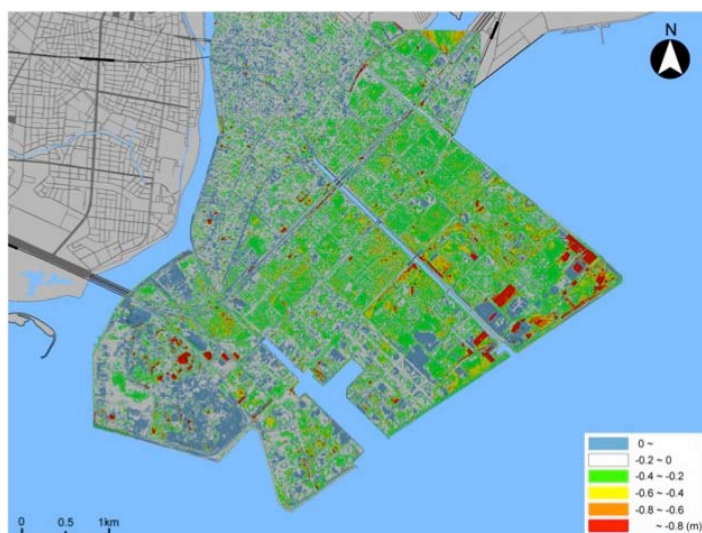
Figure 4.7. Map showing vertical ground settlement between 2006 and 2011 (Tokimatsu & Katsumata, 2012)
