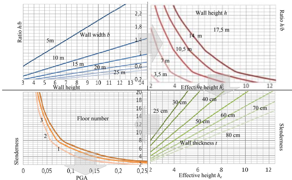
**Figure 4.1.** Nomogram for the overturning mechanisms of a wall.
