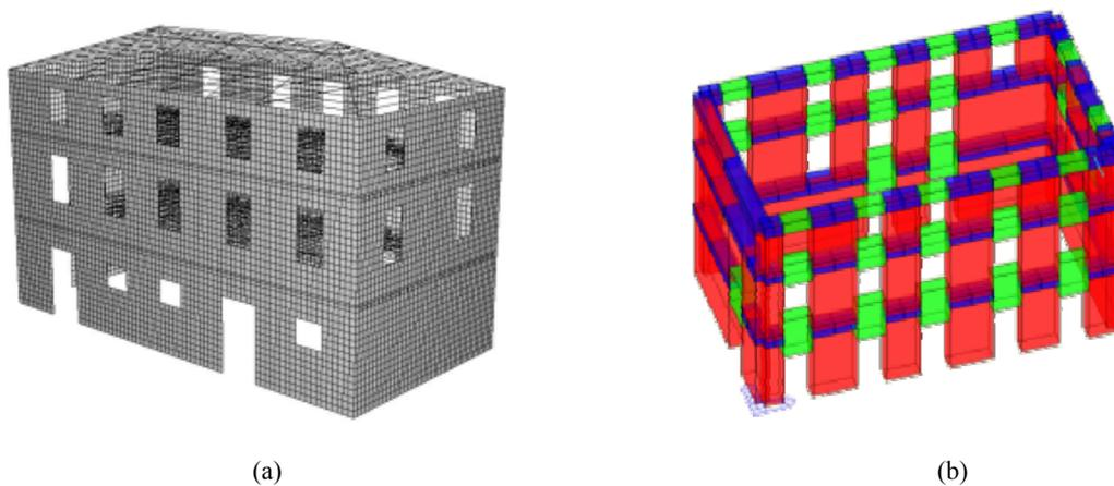
**Figure 5.1.** Numerical model for the masonry building: (a) 2D model (Abaqus), (b) equivalent frame model (MidasGen).
