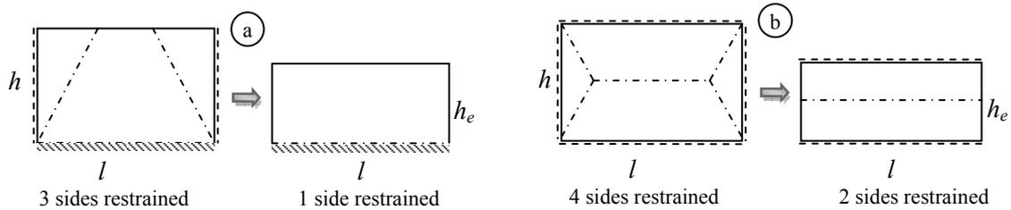
**Figure 4.2.** Collapse mechanisms for real and equivalent walls: a) real wall with 3 sides restrained equivalent to a wall with fixed end at the bottom, b) real wall with 4 sides restrained equivalent to a wall with hinges at both ends.
