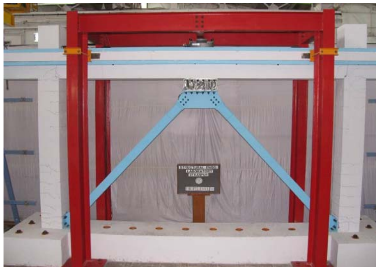
Figure 3.1 Test frame at the conclusion of the testing program showing yielded and buckled ALSYD-2 unit and minor flexural cracking in frame members
