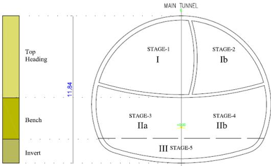
**Figure 2.** Excavation stages of main tunnel support (TETCO, 2011)
