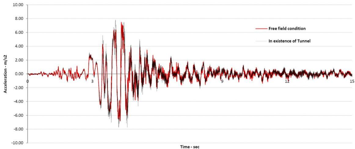
**Figure 7.** Computed acceleration time history at selected target point at top of tunnel (point B)
