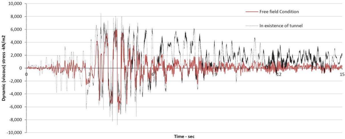
**Figure 8.** Computed Dynamic stress time history at selected target point in surface (Point A)
