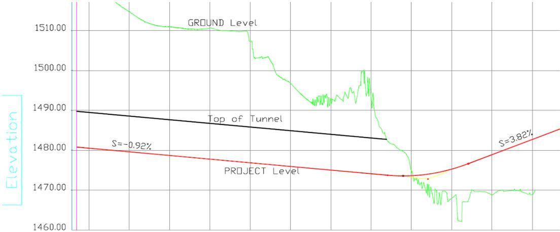
**Figure 3.** Profile of tunnel in lowest overburden location (TETCO, 2011)
