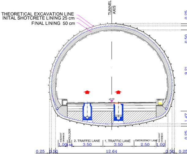
**Figure 1.** Cross section of main tunnel (TETCO, 2011)
