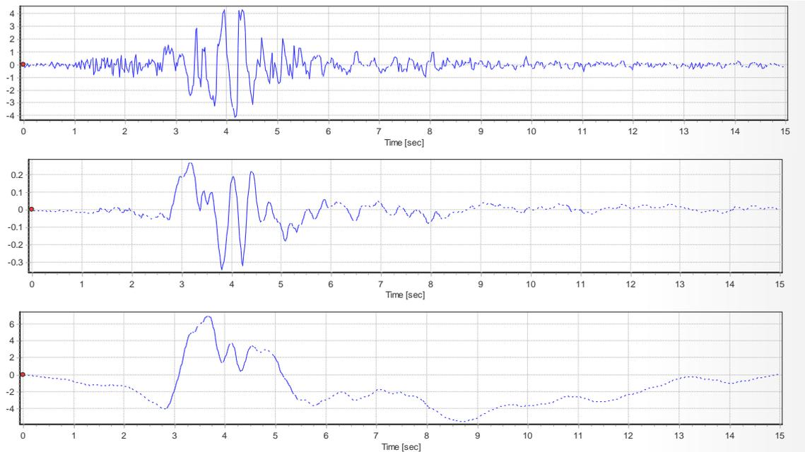
**Figure 5.** The corrected acceleration with velocity and displacement related to Loma Prieta earthquake
