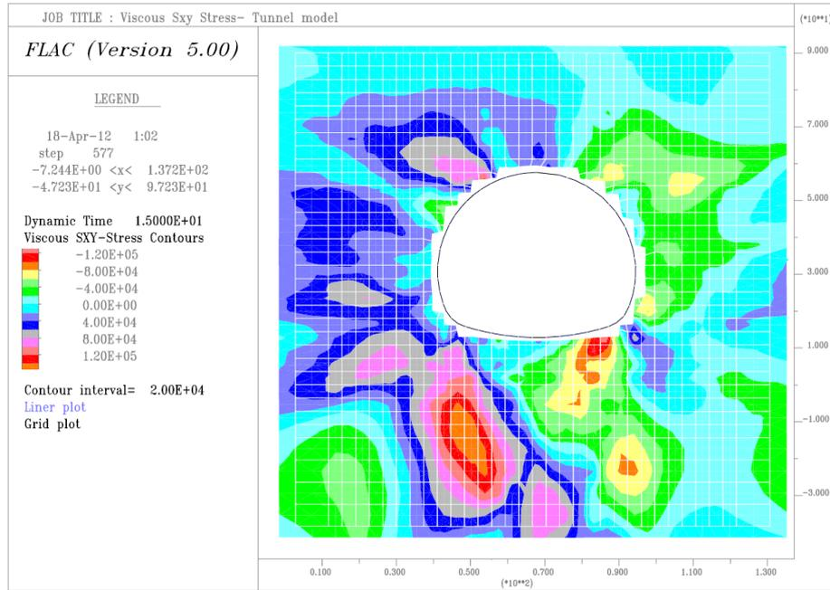
Figure 10. Dynamic stress contour in t=15 sec, Tunnel model
