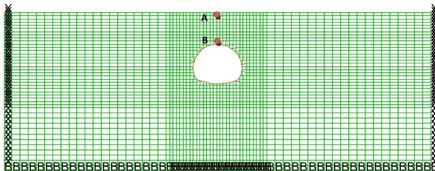
**Figure 4.** Geometry of model and mesh generation with target points
