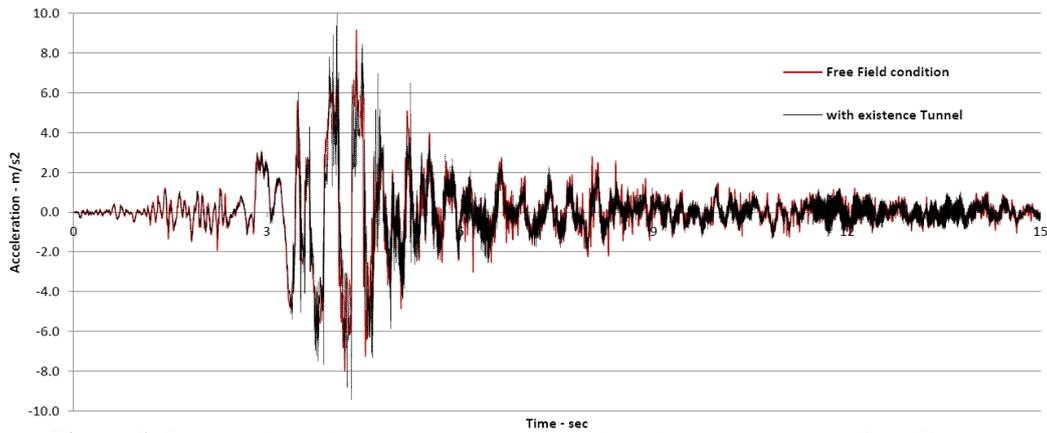
**Figure 6.** Computed acceleration time history at selected target point in surface (Point A)
