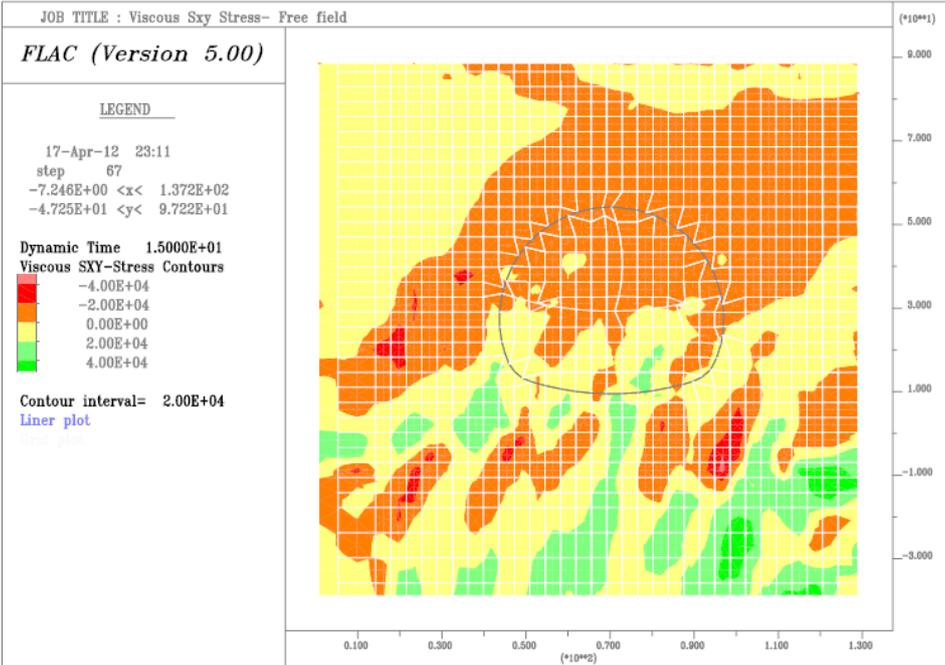
**Figure 9.** Dynamic stress contour in t=15 sec, free field model
