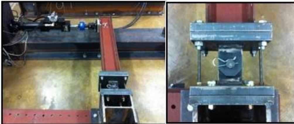
**Figure 2.** The nonlinear SDOF system that consists of a hydraulic actuator, a steel loading beam, a pin connection, two steel rods, and low-friction wheel.
