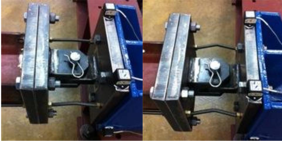
**Figure 7.** Steel rods at different stages of the effective force test series; (a) after the test with the reference force level of 6005 N and (b) after the test with the reference force level of 7562 N.
