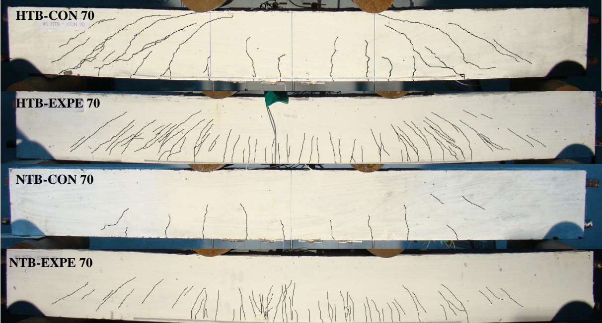
Figure 5. Failure behavior of beams
