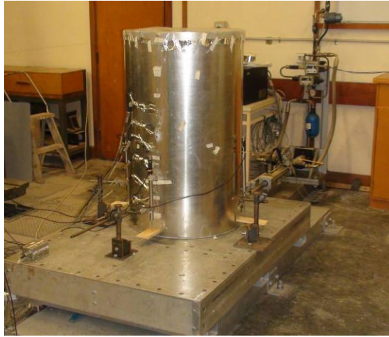
Figure 3. Experiment model made of aluminium on the shale table
