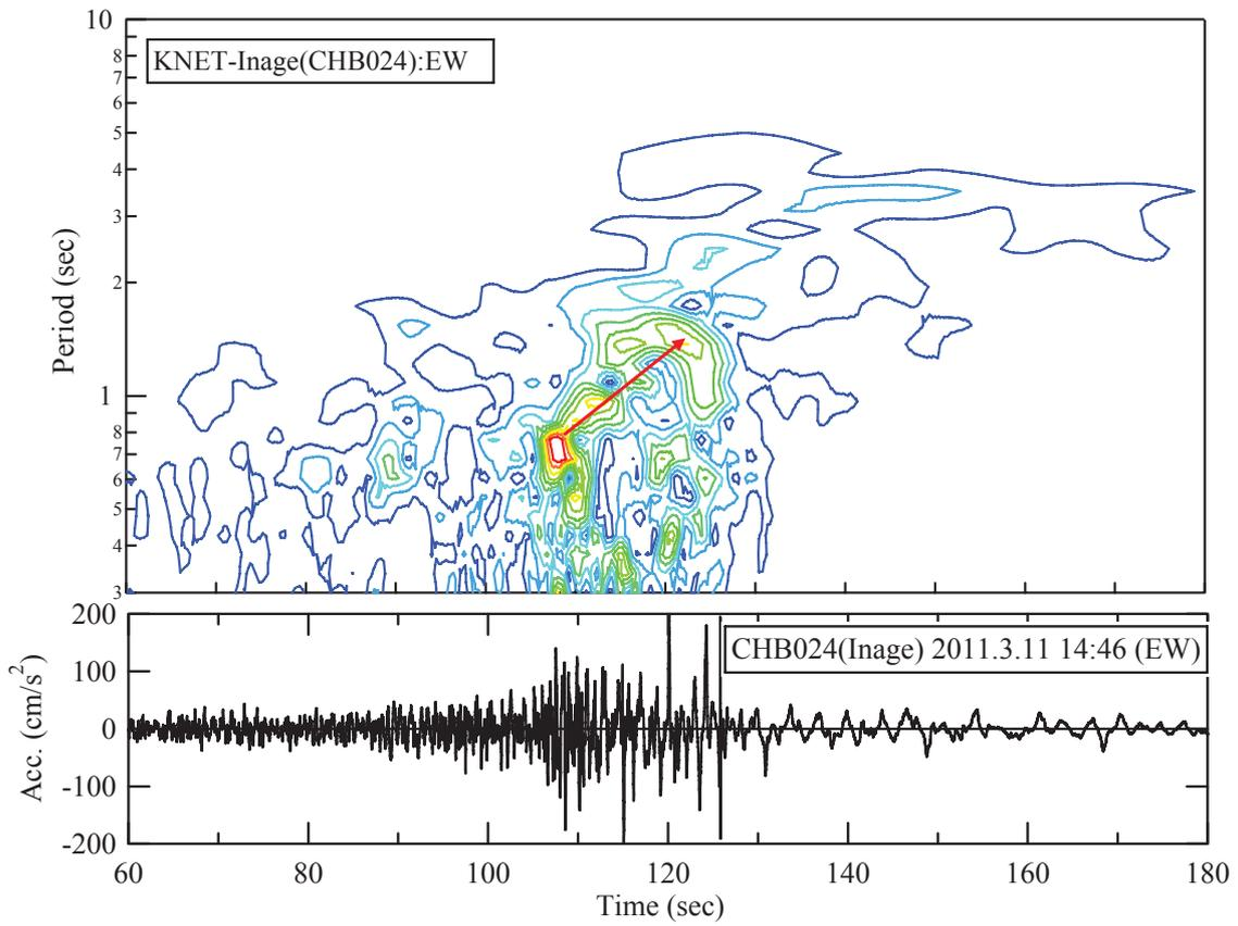
**Figure 4.4.** Non-stationary spectrum of observed record at K-NET Inage (EW comp.)
