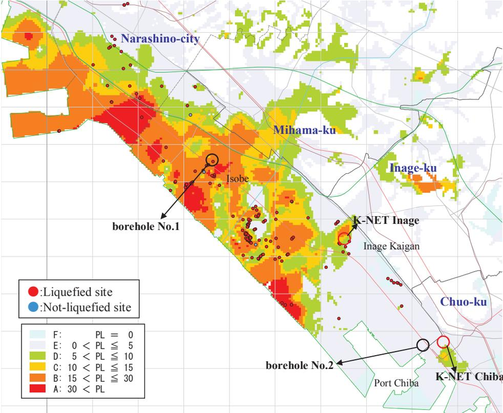
Figure 4.2. Comparison of liquefied area and estimated area during the Pacific coast of Tohoku at the coast area in Chiba city
