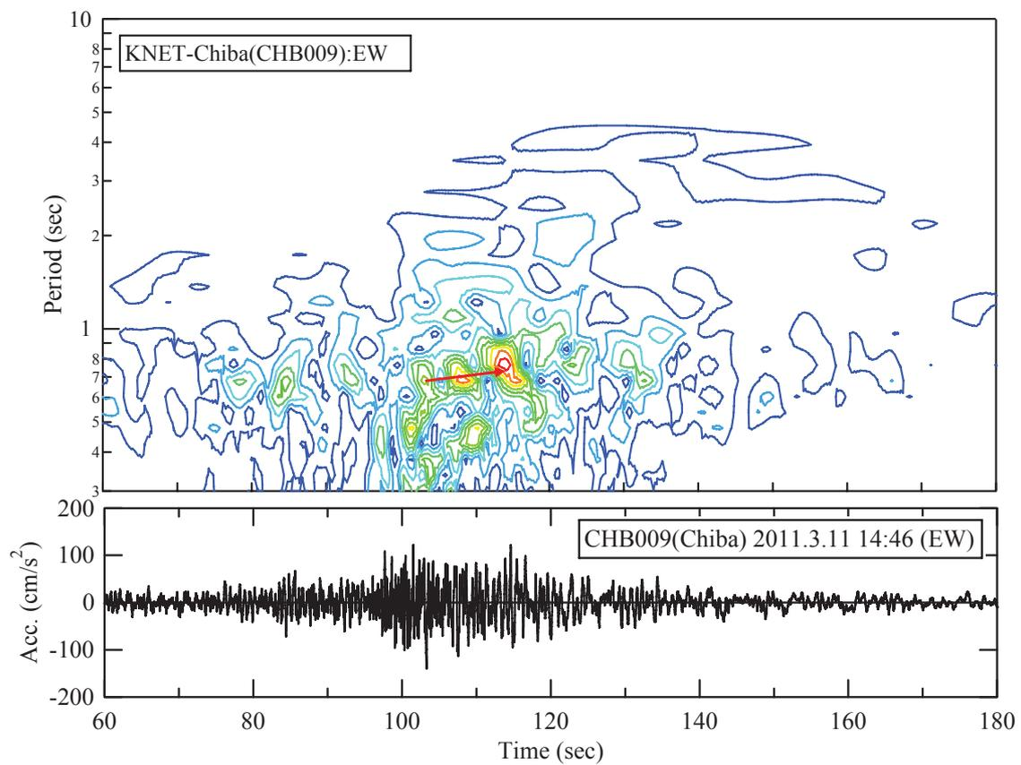
**Figure 4.5.** Non-stationary spectrum of observed record at K-NET Chiba (EW comp.)
