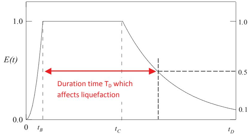
**Figure 2.1.** Duration time  $T_D$  which affects liquefaction
