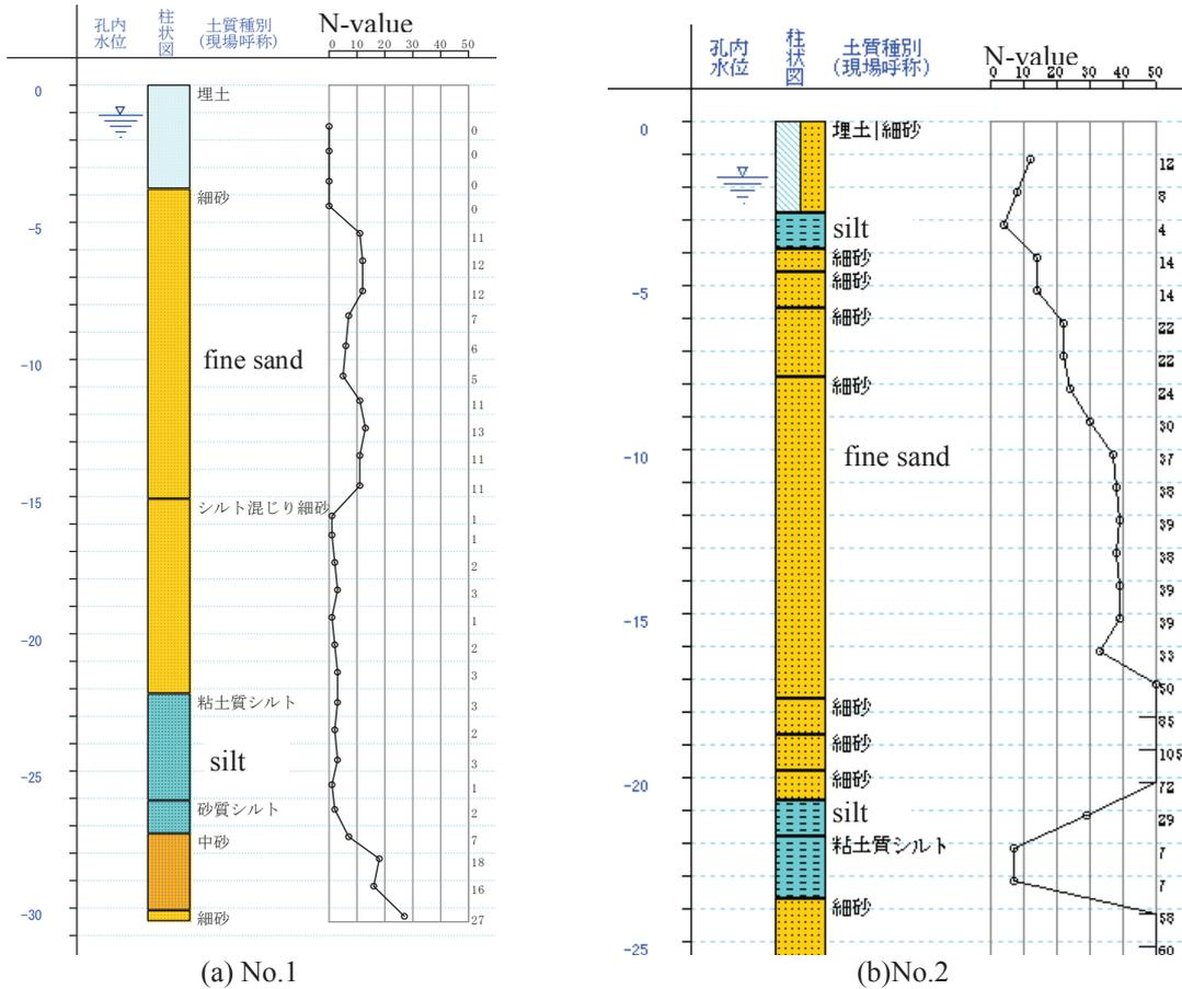
Figure 4.3. N-values and geology and by borehole data
