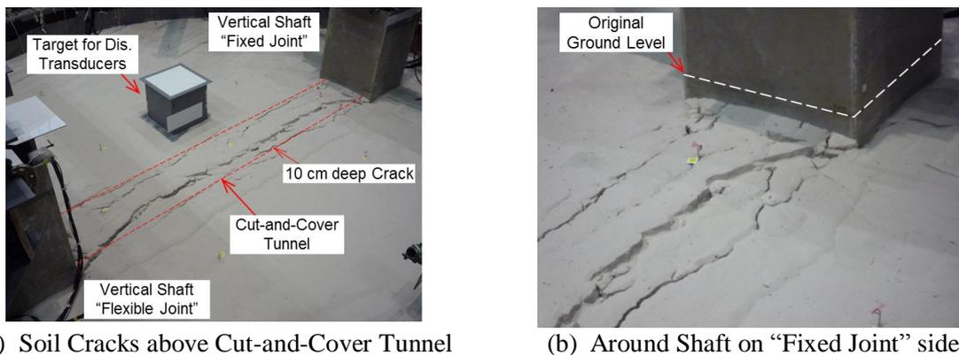
**Figure 7.** Crack and Settlement of Soil around Cut-and-Cover Tunnel
