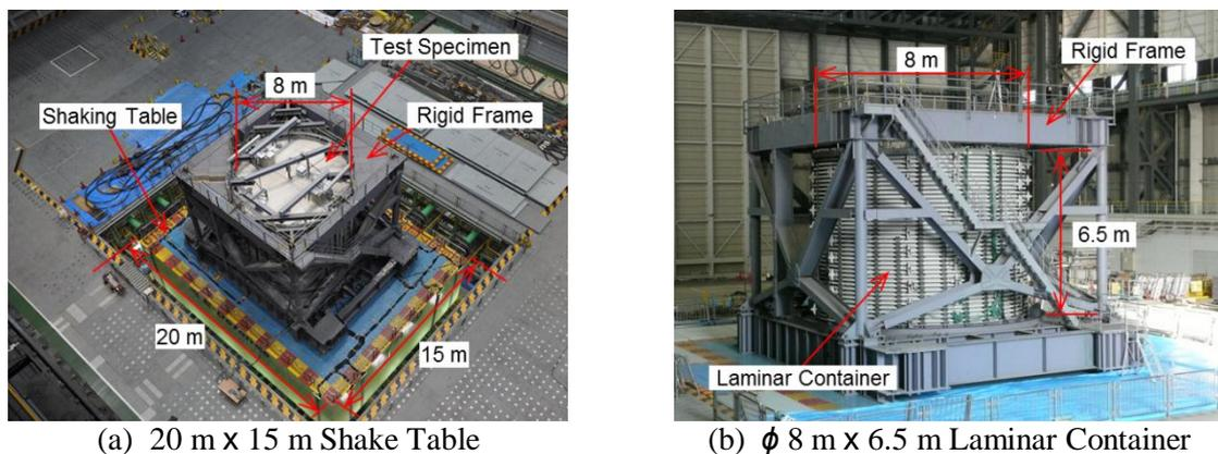
**Figure 1.** Shake Table and Soil Container
