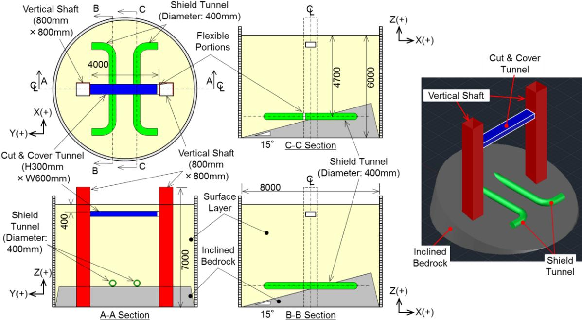
Figure 2. Setup of Test Specimen and 3-dimensional Image w/o the Container and Surface Layer
