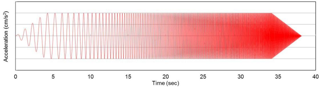
**Figure 3.** Step Sine Motion (1 - 20 Hz)
