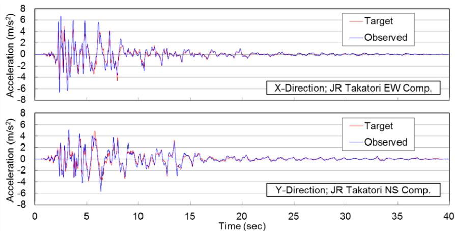
**Figure 5.** Comparison of Target and Observed Motions, Acc. Time Histories, JR Takatori 80%
