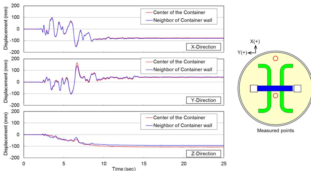
**Figure 11.** Displacement Time Histories of Ground Surface
