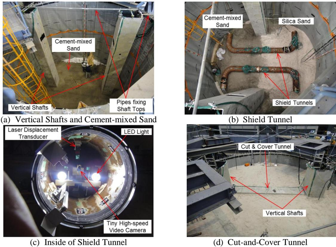
**Figure 4.** Construction of Test Specimen
