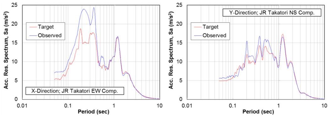
**Figure 6.** Comparison of Target and Observed Motions, Acc. Response Spectrum, JR Takatori 80%
