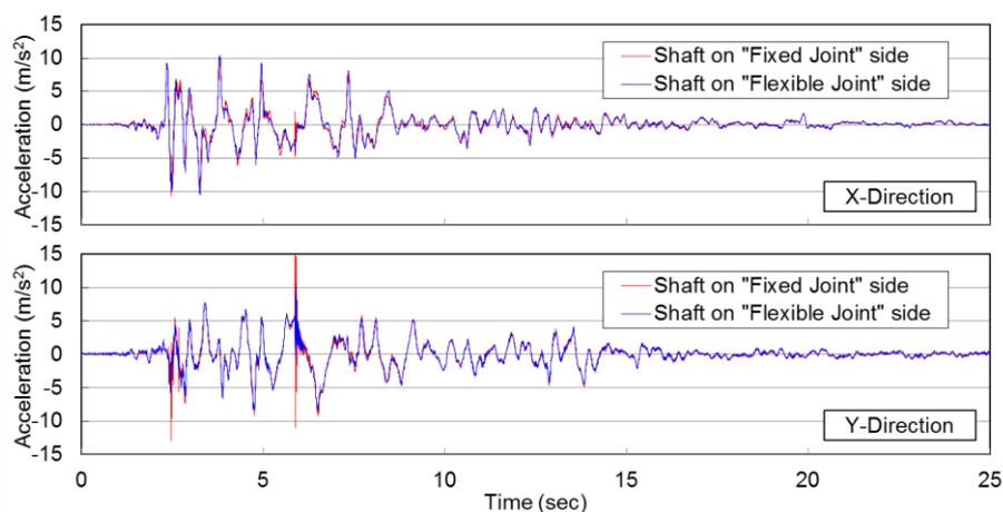
**Figure 12.** Acceleration Time Histories at Tops of Shafts
