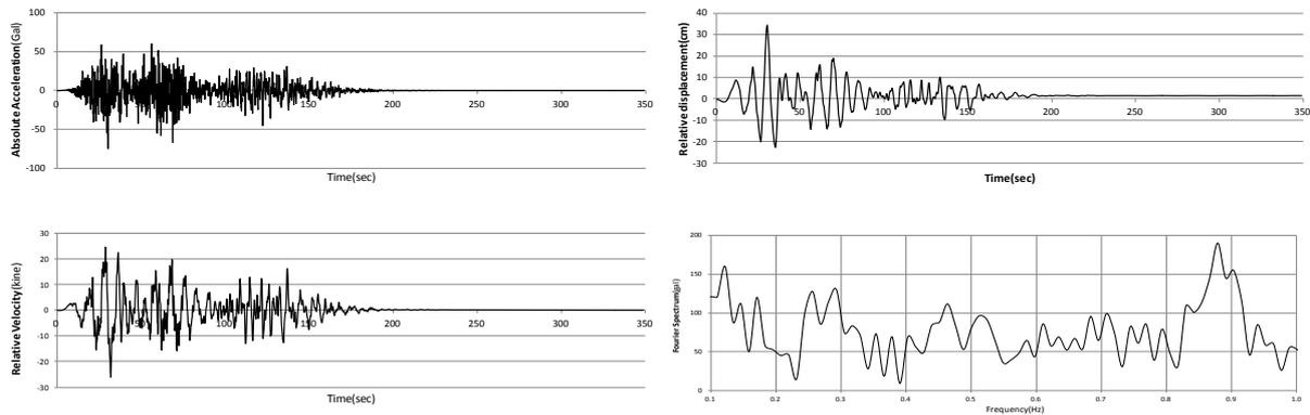
Time History Waveforms and Spectrum of the Possible Earthquake Ground Motion (OSKH02)
