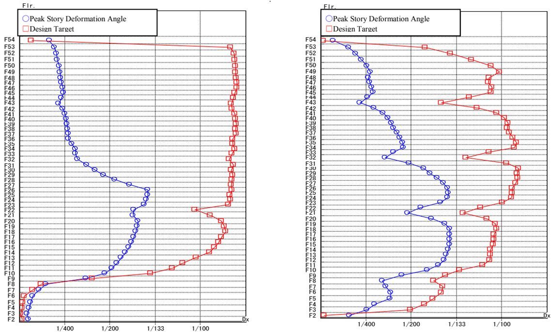
**Figure 15.** Peak Story Deformation Angle of Each Story with Damping Constant 5.0%.
