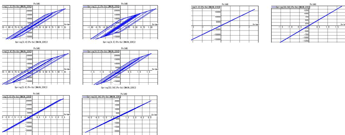
**Figure 9.** Story Shear Force: Story Deformation Charts with Damping Constant 5.0%
