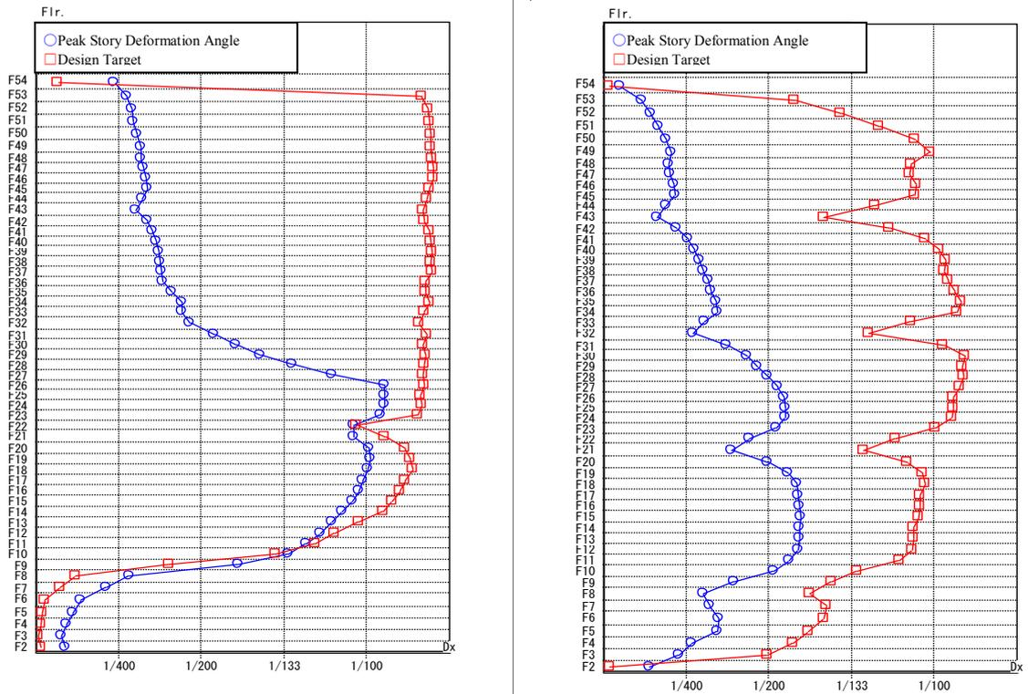
**Figure 5.** Peak Story Deformation Angle of Each Story (Left:229 Right:319)
