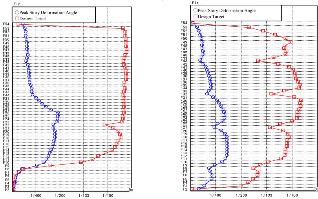
**Figure 8.** Peak Story Deformation Angle of Each Story with Damping Constant 5.0%
