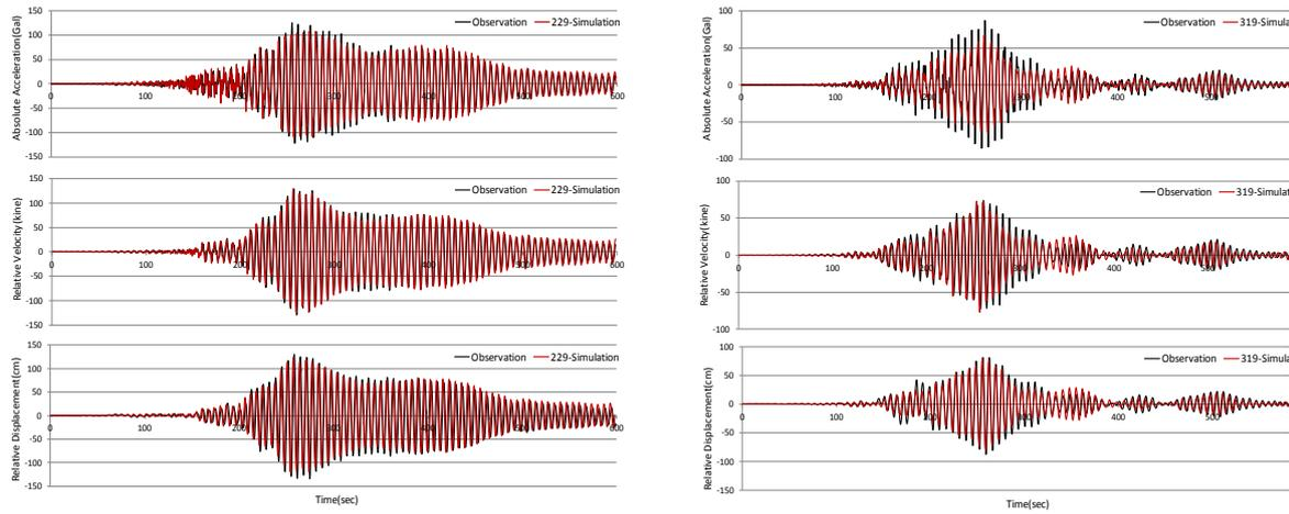
**Figure 4.** Comparison between Simulation Results from 53-DOF and Observation Records from the Tohoku-Oki Earthquake (From top, absolute acceleration, relative velocity, and relative displacement)
