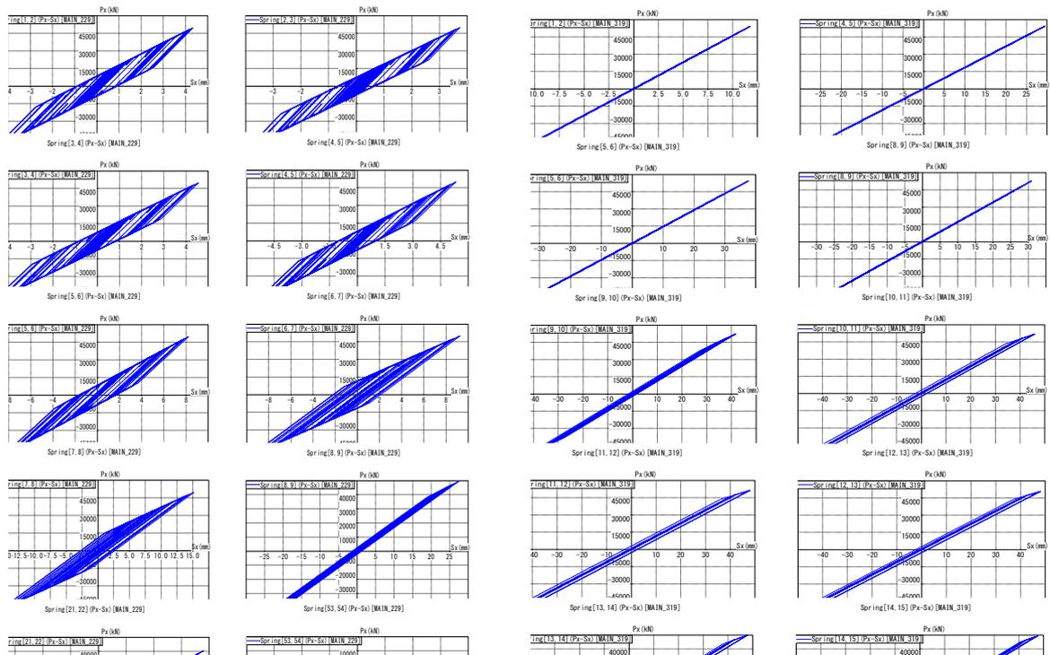
**Figure 13.** Story Shear Force of Stores Exceeded Elastic Limit versus Story Deformation Charts
