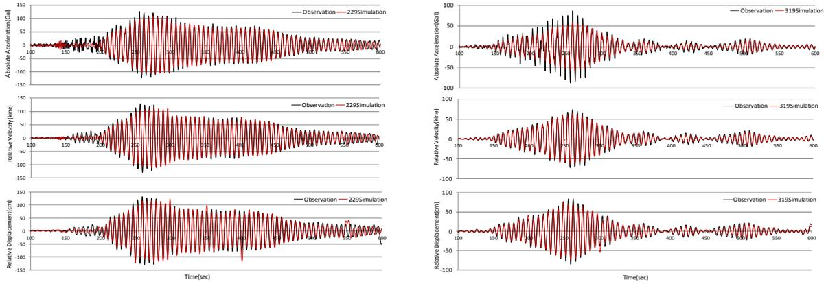
**Figure 2.** Comparison between Simulation Results from 1-DOF and Observation Records from Tohoku-Oki Earthquake
