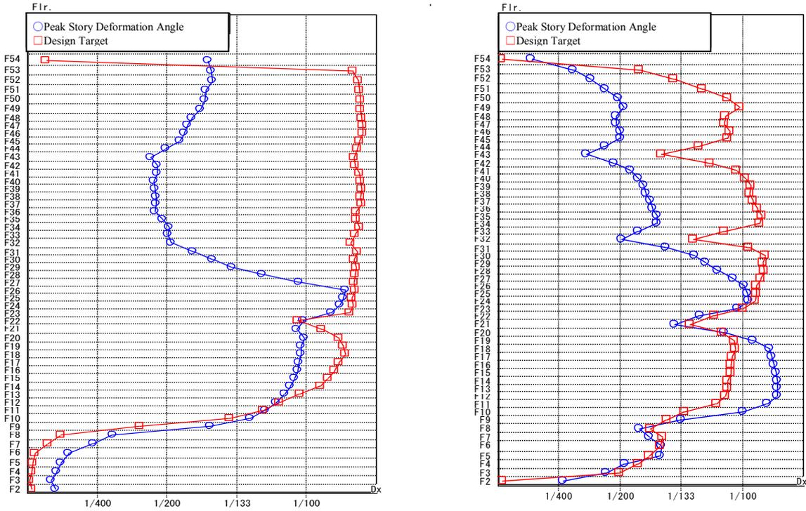
**Figure 12.** Peak Story Deformation Angle of Each Story for the Nankai Earthquake(Left:229 Right:319)
