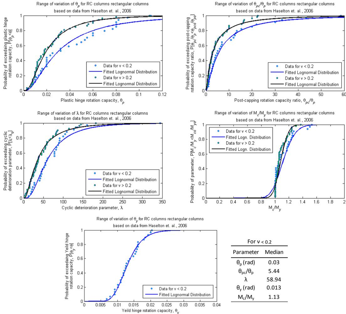
**Figure 2.** Range of variation and fitted distributions for component parameters  $M_c/M_y$ ,  $\theta_p$ ,  $\theta_{pc}/\theta_p$  and  $\lambda$  utilized in modified Ibarra-Krawinkler deterioration model for two axial load intensities  $v$ , based on data from Haselton et. Al. 2006 and selected median values for the three cases
