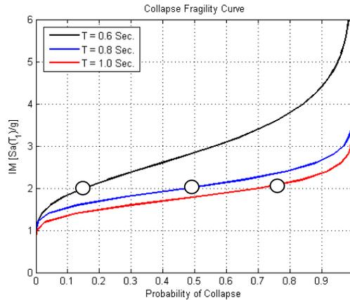
**Figure 5.** Collapse fragility curves of all 4-Story 2D RC Frames based on IDA of the buildings under FEMA P-695 Far Field Ground Motion Set
