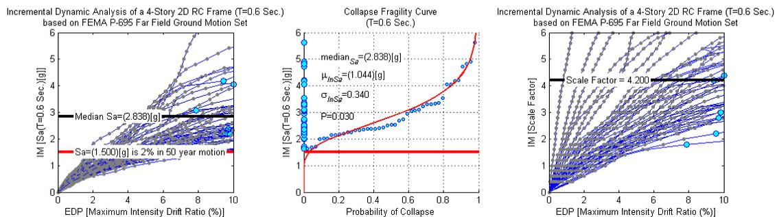
**Figure 4.** Incremental Dynamic Analysis of a 4-Story 2D RC Frame (T=0.6 Sec.) based on FEMA P-695 Far Field Ground Motion Set
