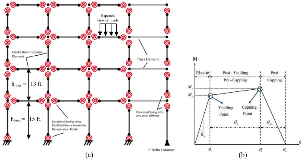
**Figure 1.** Schematic concentrated plasticity OpenSees model of 4-story RC-SMRF structural analysis model (a), Backbone curve definition based on typical modified Ibarra-Krawinkler deterioration model where  $K_e$  is the initial stiffness,  $M_y$  is the yield moment,  $M_c/M_y$  is the capping moment ratio,  $\theta_p$  is the plastic hinge rotation capacity, and  $\theta_{pc}/\theta_p$  is the post-capping rotation capacity ratio (b)
