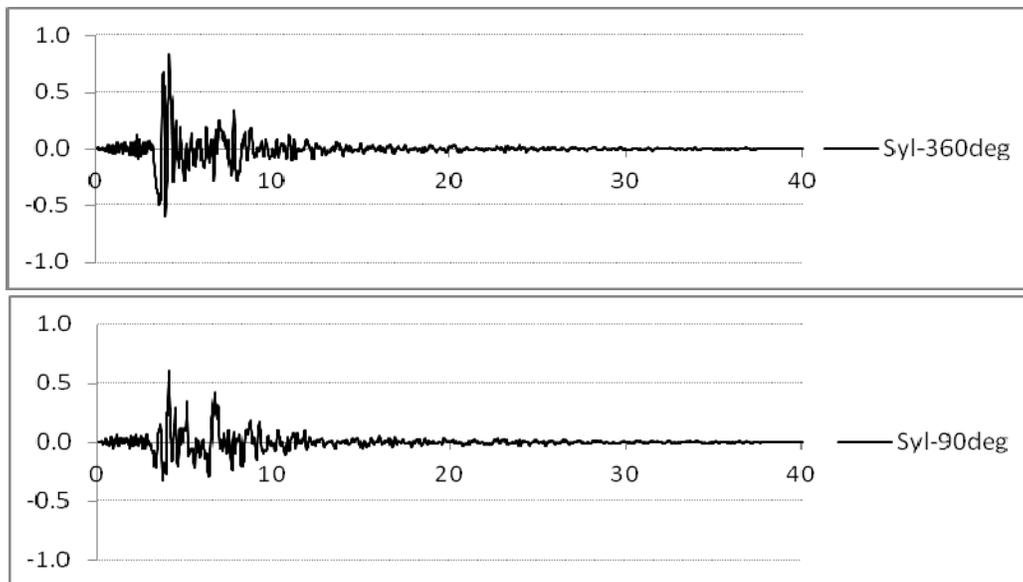
**Figure 5.** Acceleration time histories of Northridge earthquake recorded at Sylmar station in both directions
