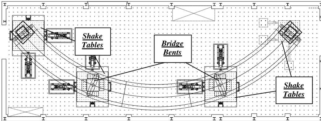
**Figure 9.** Plan view of the laboratory including the bridge
