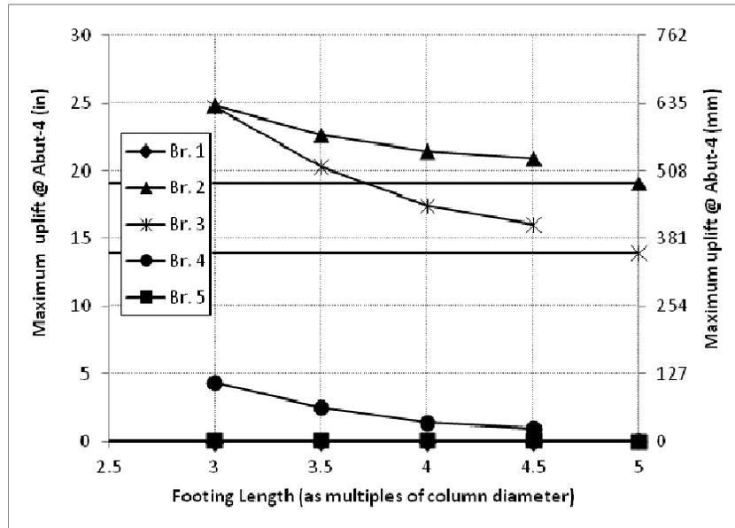
Figure 8. Maximum displacement in the first abutment vs. footing size for the 300% DE level
