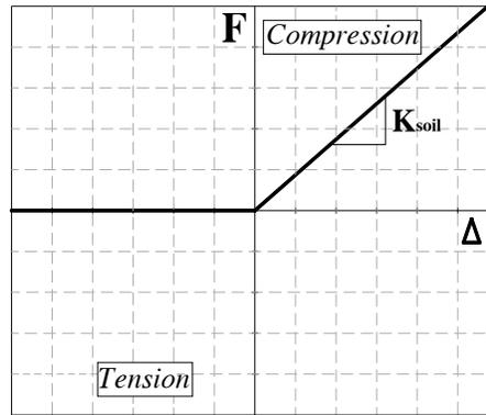
**Figure 4.** Force-displacement relationship for the gap elements used in defining the soil springs
