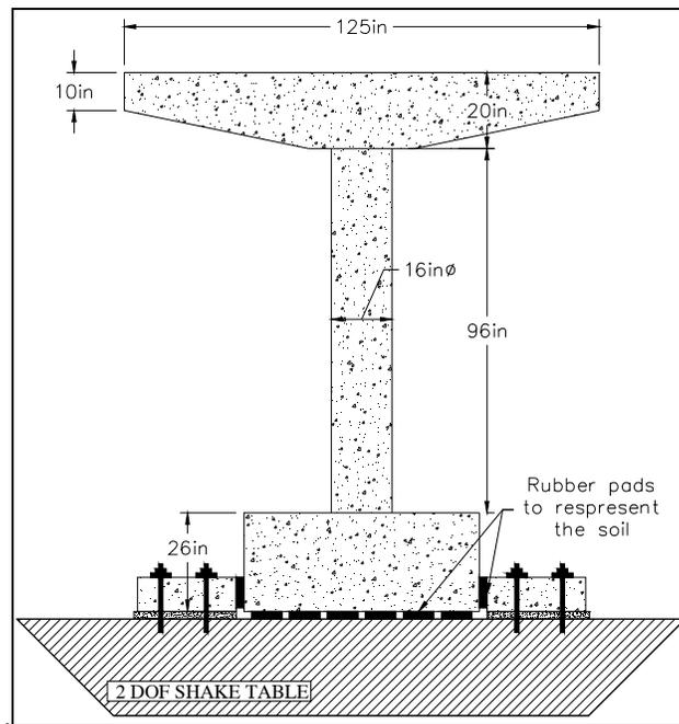
**Figure 10.** Experimental setup for the bridge pier
