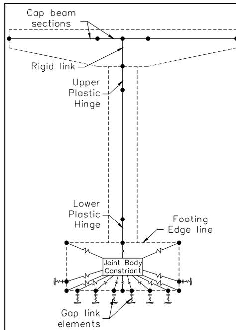
**Figure 3.** Modeling of the pier elements in SAP2000
