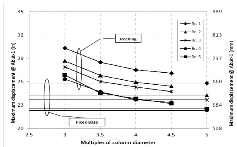
**Figure 7.** Maximum displacement in the first abutment vs. footing size for the 300% DE level
