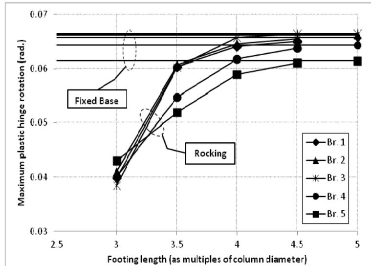
**Figure 6.** Maximum plastic hinge rotation in the lower hinge of the first pier column vs. footing size for the 300% DE level
