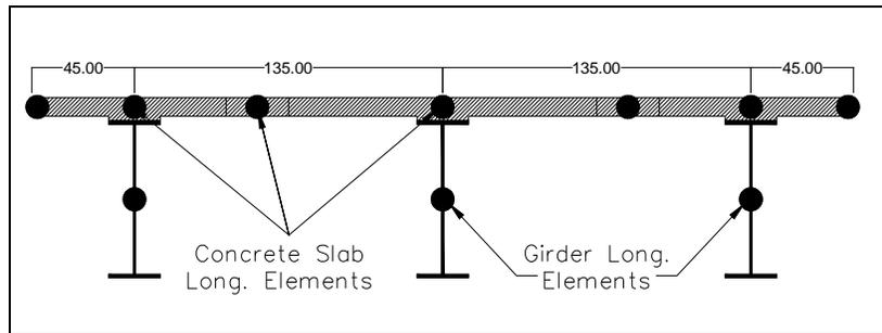
**Figure 2.** Bridge cross section with the locations of the longitudinal elements used in the analytical models
