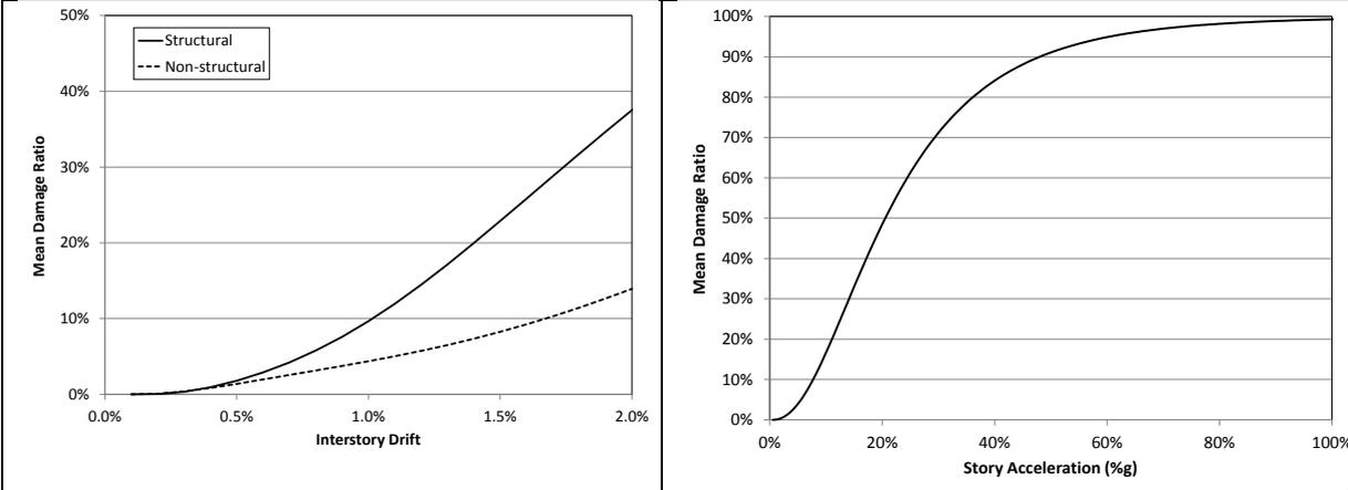
**Figure 5.** Story damage function for estimating structural and non-structural drift-sensitive damage (left) and non-structural acceleration sensitive damage (right) of the case-study building.
