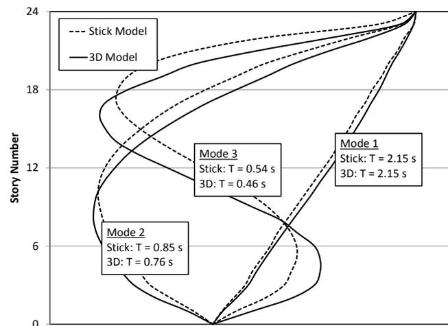
**Figure 4.** First three elastic mode shapes and corresponding periods for the 3D model and the stick model.
