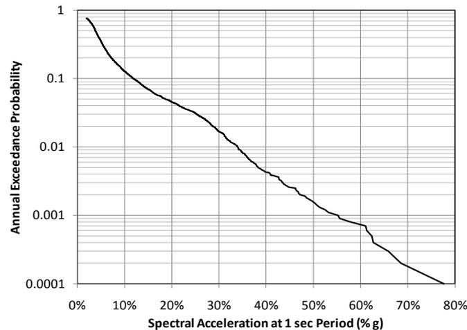
**Figure 1.** Probabilistic hazard curve for the case study building.
