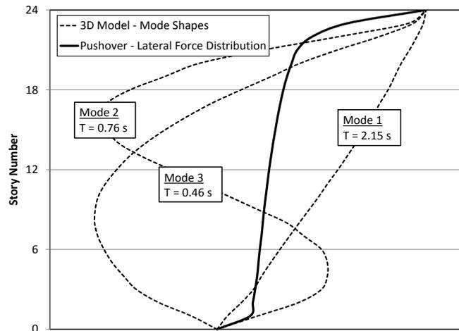
**Figure 2.** Comparison between the first three mode shapes in the longitudinal direction of the three-dimensional model and the lateral force pattern for the pushover analysis.
