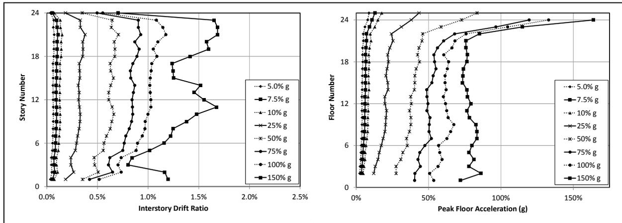
**Figure 3.** Distribution of median interstory drift (left) and median absolute floor acceleration (right) from IDAs.
