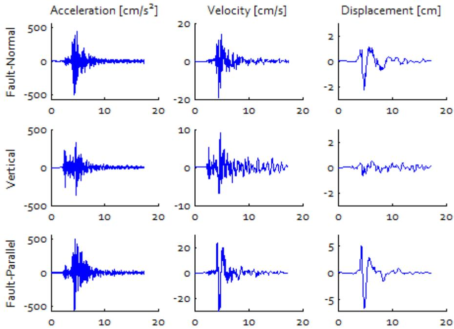
**Figure 5.** Corrected acceleration, velocity, and displacement time histories of the strike-parallel, strike-normal, and up-down components of strong motion records
