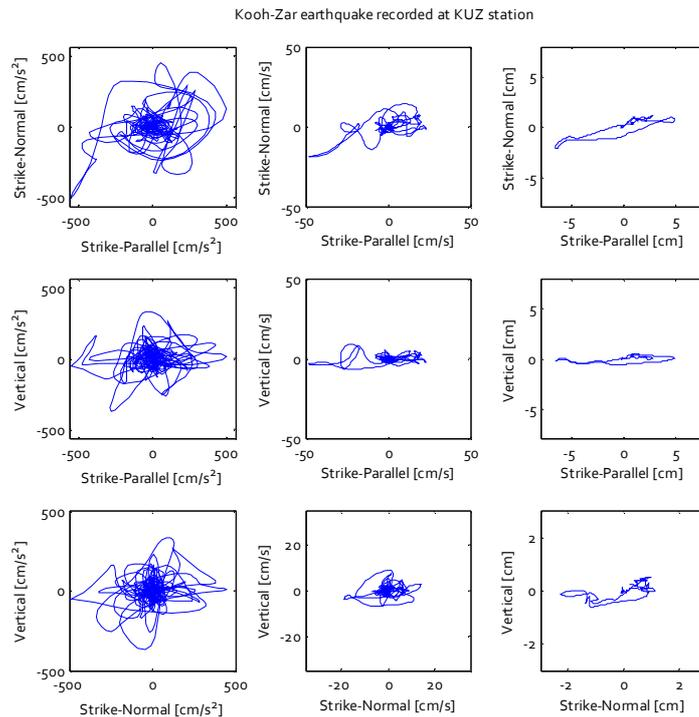
**Figure 6.** Acceleration, velocity, and displacement particle motions
