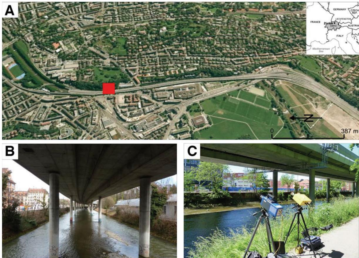
**Figure 1.** A) Sihlhochstrasse bridge test site: the red box highlights the location of measurements; B) piles in river Sihl; C) FLIR (on the left) and IBIS-S (on the right) sensors during acquisition.
