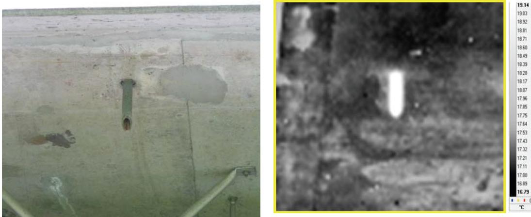
**Figure 2.** Left, example of a frame acquired by FLIR camera. The frame depicts a metal object (nut) solidly connected to the bridge structure that was used as a target to observe the thermal oscillation caused from the heavy vehicles traffic on the bridge. Right, the FLIR acquisition area used for calculating the oscillation frequencies.
