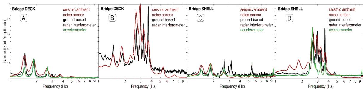
**Figure 5:** Comparison between the Fourier spectra obtained for the horizontal and vertical component of the deck (A, B) and the shell (C, D) oscillations of the Musmeci Bridge by using the three different sensors, in the frequency band 1 – 10 Hz. The ground-based radar interferometer results are indicated with a black line, while red lines and green lines represent those obtained by the seismic ambient noise sensor and the accelerometer, respectively.
