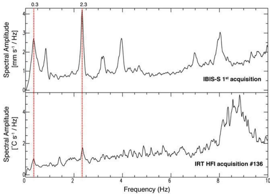
**Figure 3.** Comparison between the velocity Fourier spectrum obtained from the IBIS-S data (1st acquisition) and the Fourier spectrum obtained from the derivative of the FLIR camera data. Red dotted lines indicate the resonant frequencies commonly identified by both the sensors. These frequencies are related to purely vertical oscillations of the Sihllochstrasse Bridge.
