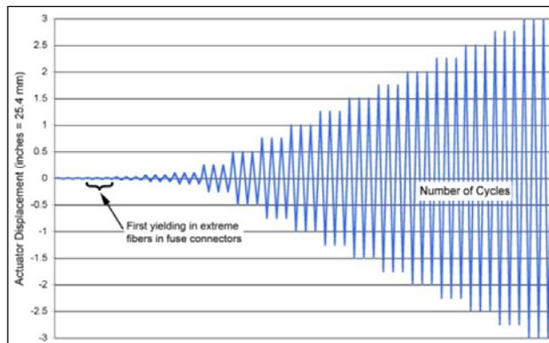
**Figure 4.** Modified ATC-24 Cyclic Loading Routine.
