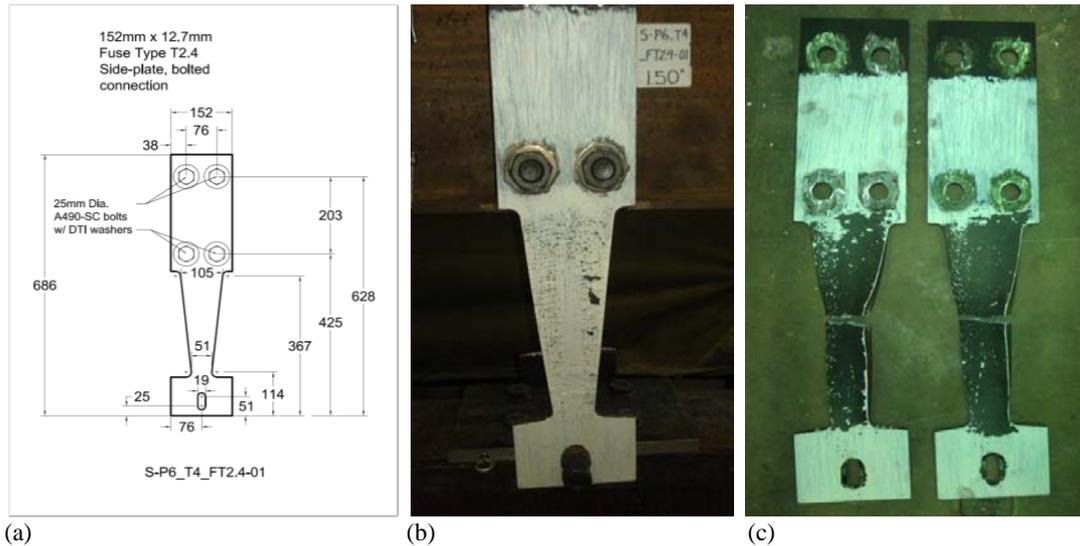
**Figure 5.** Typical 6" Fuse Plate: (a) schematic; (b) during test; (c) after failure.
