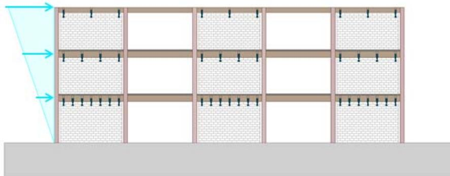
**Figure 9.** Sample Distribution of Fuse Plates within Single Building Frame.
