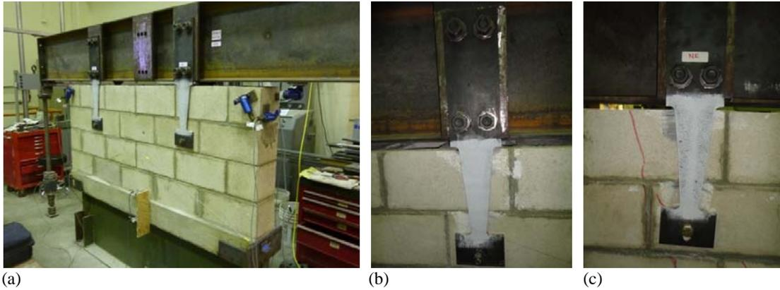
**Figure 2.** Tapered Fuse Test Specimen: (a) test setup; (b) fuse detail pre-test; (c) fuse detail post-test.
