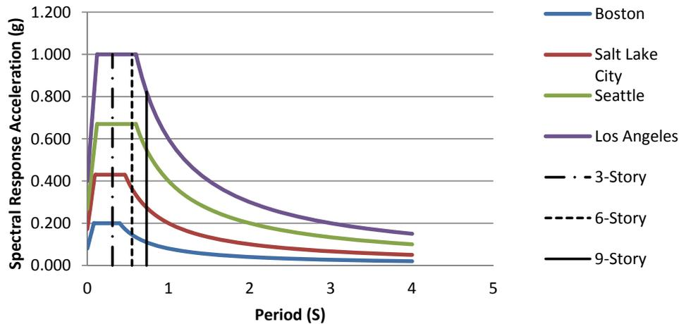
**Figure 8.** Design Response Spectra with Approximate Periods.
