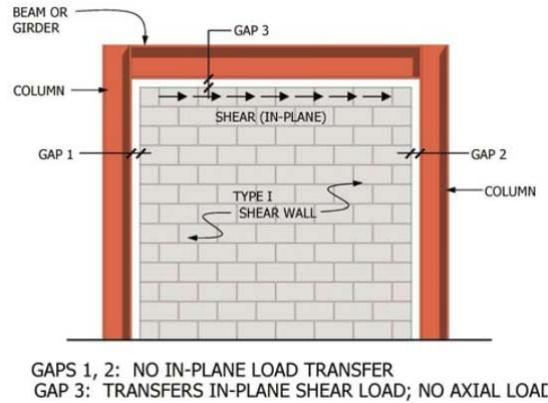
**Figure 1.** Type I Hybrid Wall [NCMA 2009].
