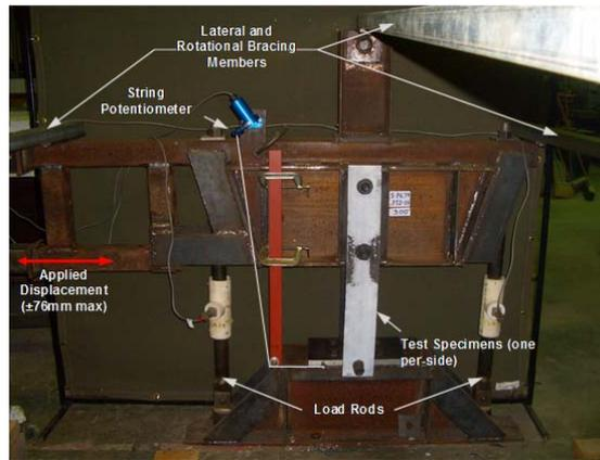
**Figure 3.** Connector and Fuse Plate Development Testing.
