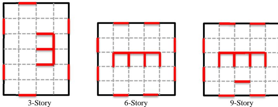
**Figure 10.** Los Angeles Prototype Plans with Hybrid Masonry Panel Locations.
