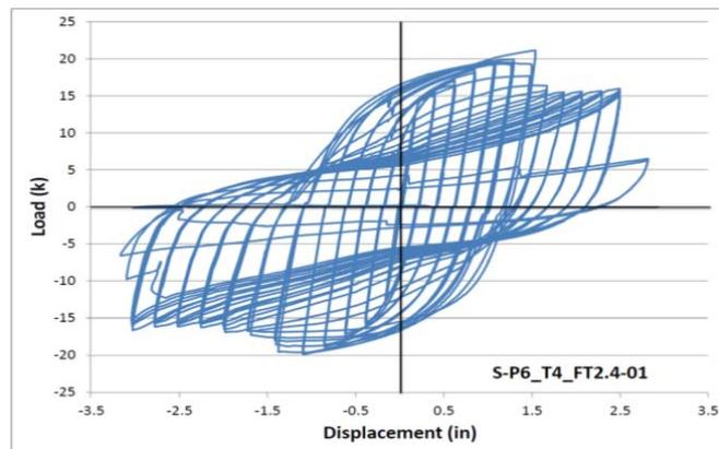
**Figure 6.** Hysteretic Response for Single Pair of 6" Tapered Fuses.
