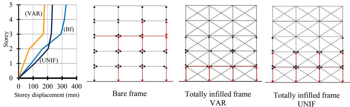
**Figure 6.4.** Displacement profiles and distribution of plastic hinges at collapse condition “b” for the accelerogram S1
