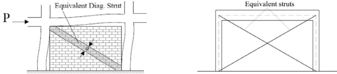
**Figure 2.1.** Equivalent diagonal struts
