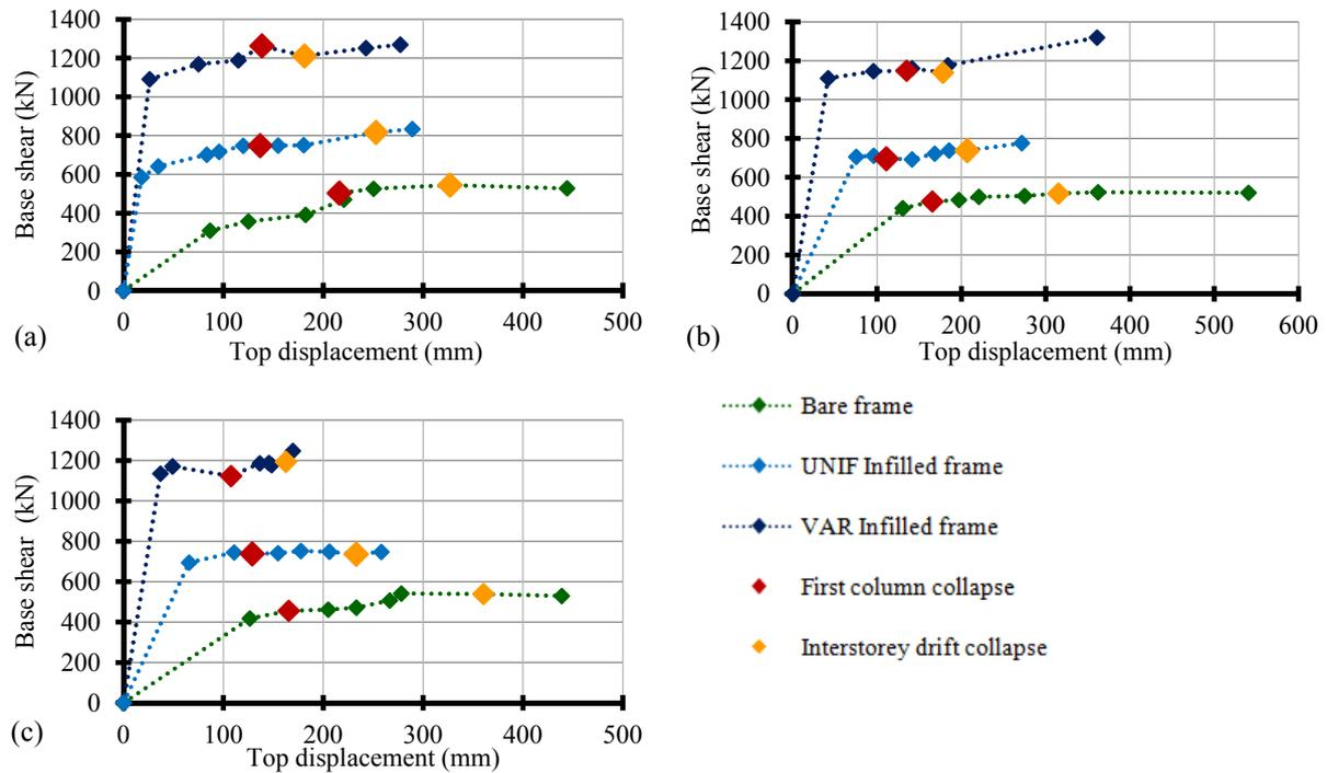
**Figure 6.3.** Top displacement-base shear curves from incremental dynamic analyses: S1 (a), S2 (b), S3 (c)
