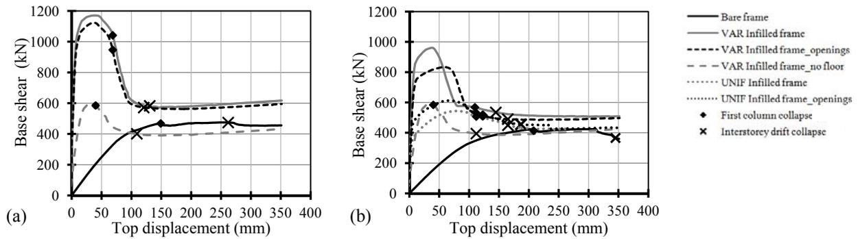
**Figure 6.1.** Pushover curves obtained with forces proportional to masses (a) and to the first mode (b)
