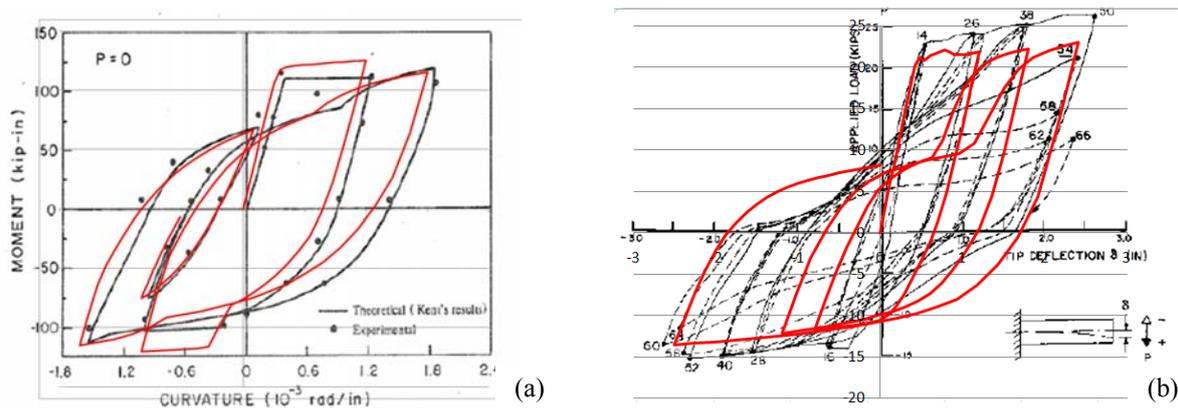
**Figure 3.1.** Analytical results compared to the experimental ones by Kent (1969) (a) and by Ma et al. (1976) (b)
