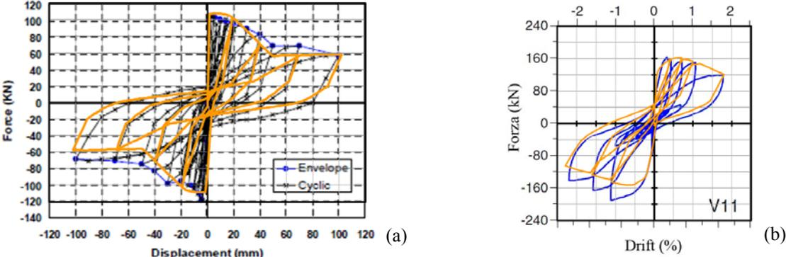
**Figure 3.4.** Numerical results for cyclic loading (orange curve) compared with the experimental results (blue curve) of Pires (1990) (a) and of Colangelo (2004)(b)
