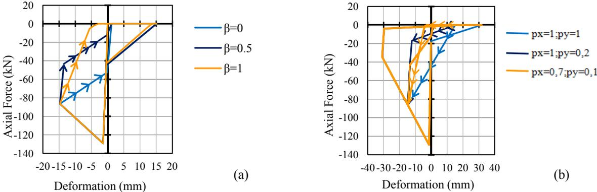
**Figure 3.3.** Strut response modified by the variation of the parameter  $\beta$  (a) and of the parameters  $p_x$  and  $p_y$  (b)
