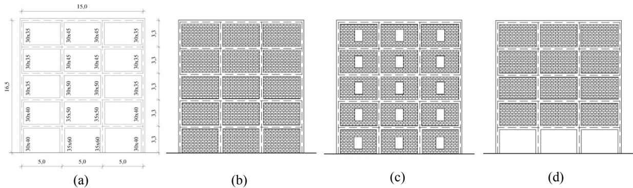
**Figure 4.1.** Representation of the examined frames: bare frame (a), totally infilled frame (b), totally infilled frame with openings (c) and infilled frame without panels at the ground floor (d)
