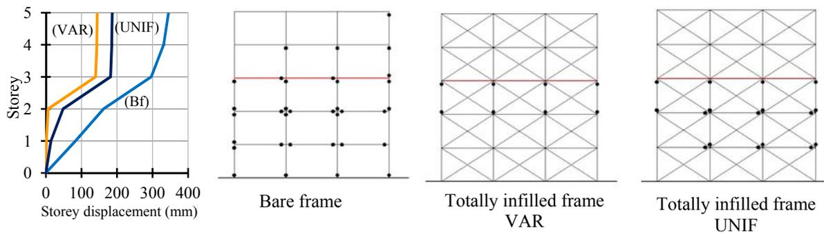
**Figure 6.2.** Displacement profile and distribution of plastic hinges at the collapse condition “b” (achievement of the ultimate interstorey drift) in the case of force proportional to the first mode
