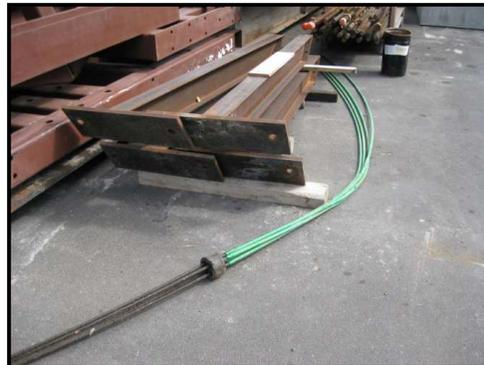
**Figure 11: Removed Tendon (After Testing)**
