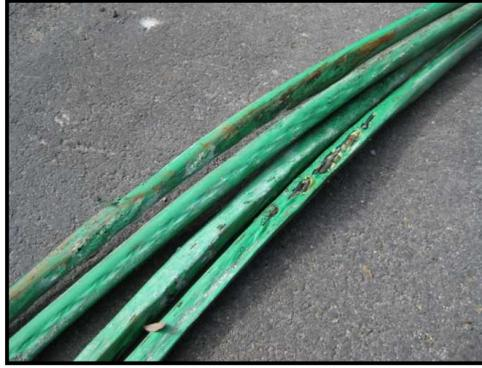
**Figure 12:** Removed Tendon at Bend in Location (After Testing)
