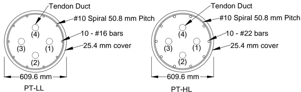
**Figure 2:** Column Cross Sections
