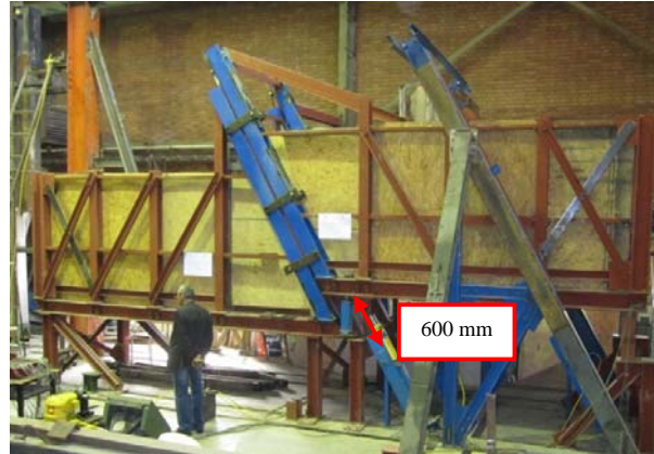
Figure 4. Split-box test basin after 600 mm faulting displacement
