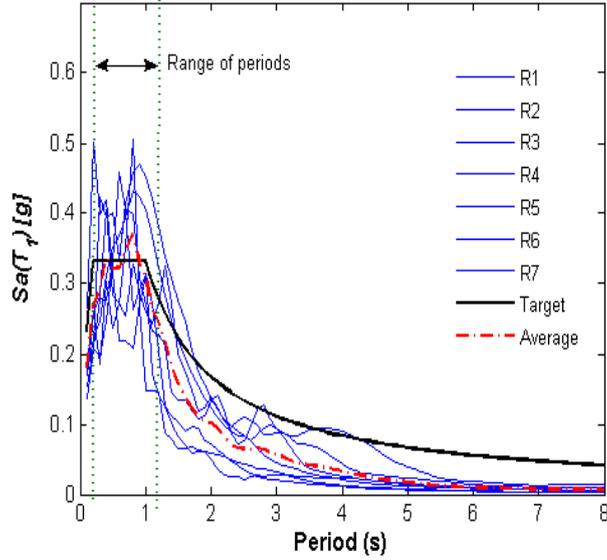
**Figure 3.3.** Set of seven earthquake response spectra obtained with the  $N_p$ -based approach and comparison among the average and the target spectra
