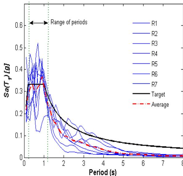
**Figure 3.1.** Set of seven earthquake response spectra obtained with the traditional approach and comparison among the average and target spectra
