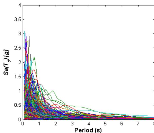
**Figure 2.1.** Elastic response spectra for the 1024 records under consideration obtained for 5% of critical damping
