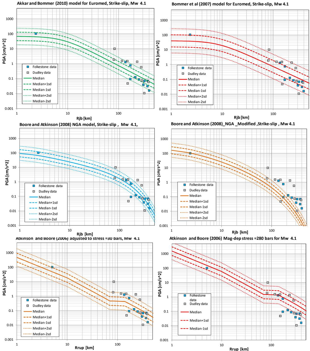
**Figure 3.** Comparison of data recorded during the Folkestone ( $M_w=4.1$ ) earthquake with median PGA values at rock predicted by the GMPEs by Akkar and Bommer (2010) and Bommer et al. (2007) for shallow crustal European and Middle East events, Boore and Atkinson (2008) NGA and Boore and Atkinson (2008 / 2011) modified for shallow crustal events and Atkinson and Boore (2006) for stable continental ENA events.
