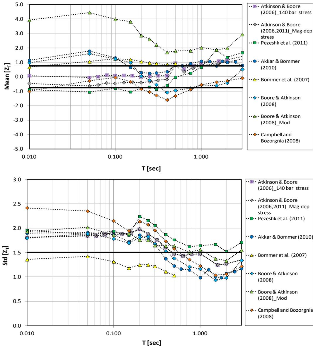
**Figure 4.** Mean normalised residuals and standard deviation of the normalised residuals (Mean  $[Z_T]$  and Std  $[Z_T]$ , respectively) across the range of spectral periods.
