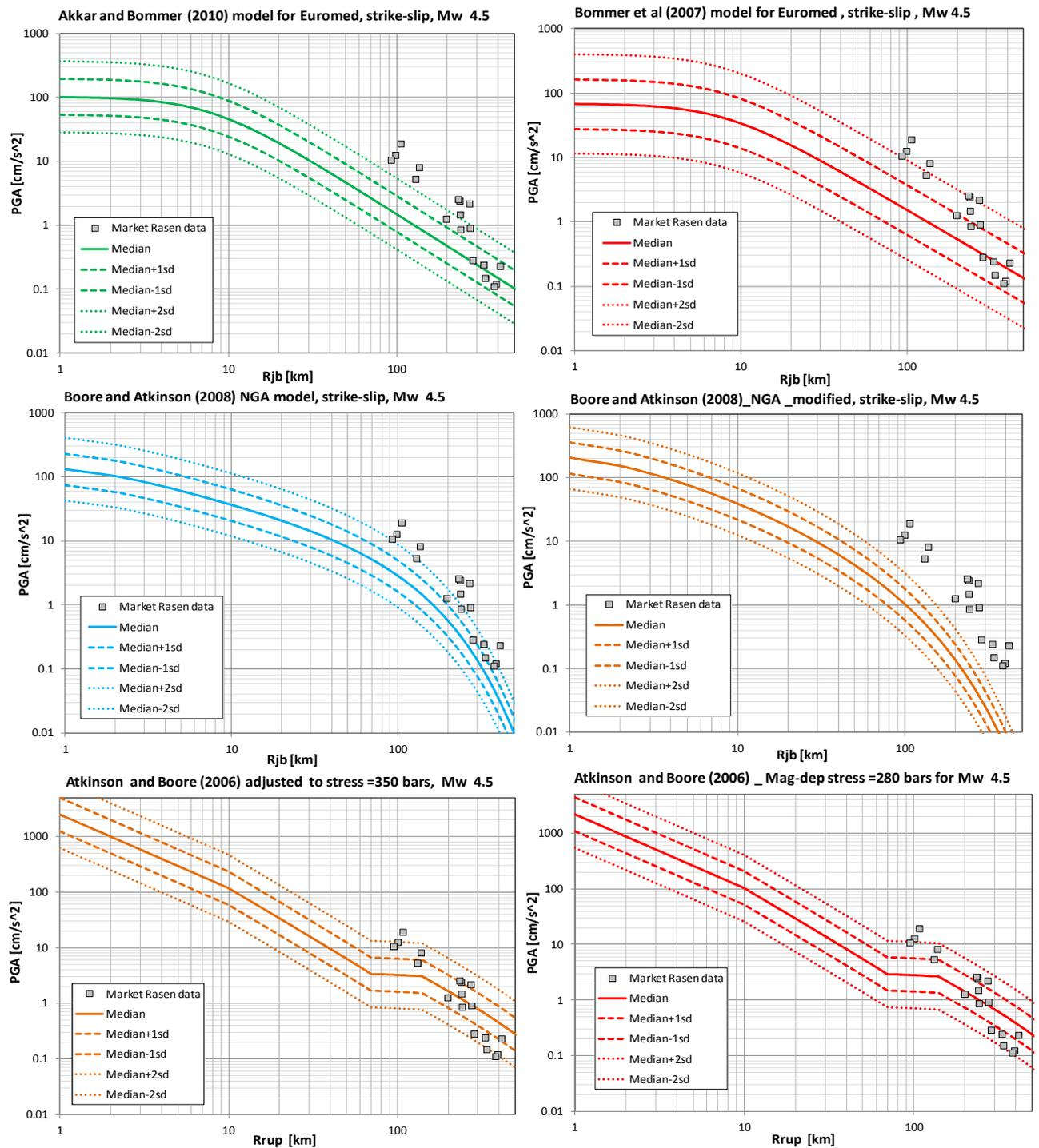
**Figure 2.** Comparison of data recorded during the Market Rasen ( $M_w=4.5$ ) earthquake with median PGA values at rock predicted by the GMPes by Akkar and Bommer (2010) and Bommer et al. (2007) for shallow crustal European and Middle East events, Boore and Atkinson (2008) NGA and Boore and Atkinson (2008 / 2011) modified for shallow crustal events and Atkinson and Boore (2006) for stable continental ENA events.
